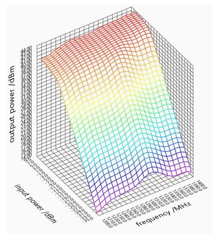
Here is the measured output power in dBm versus frequency in MHz and input power in dBm. The quiescent current at a supply voltage of 28V is 278mA.
