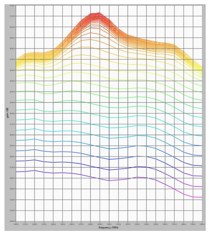
In the next picture you find the corresponding 2D graph of gain versus frequency at different input power levels:
