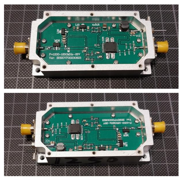
In the amplifier module the RF input signal is first amplifier by an integrated TQP3M9008 E-pHEMT MMIC amplifier from Qorvo and then boosted to the final output power level by an integrated two stage amplifier MHV5IC2215N from Freescale. In addition there are two stacked linear voltage regulators providing the 6V supply voltage to the TQP3M9008 MMIC and via two resistive dividers 5V to the biasing input of the MHV5IC2215N amplifier.
