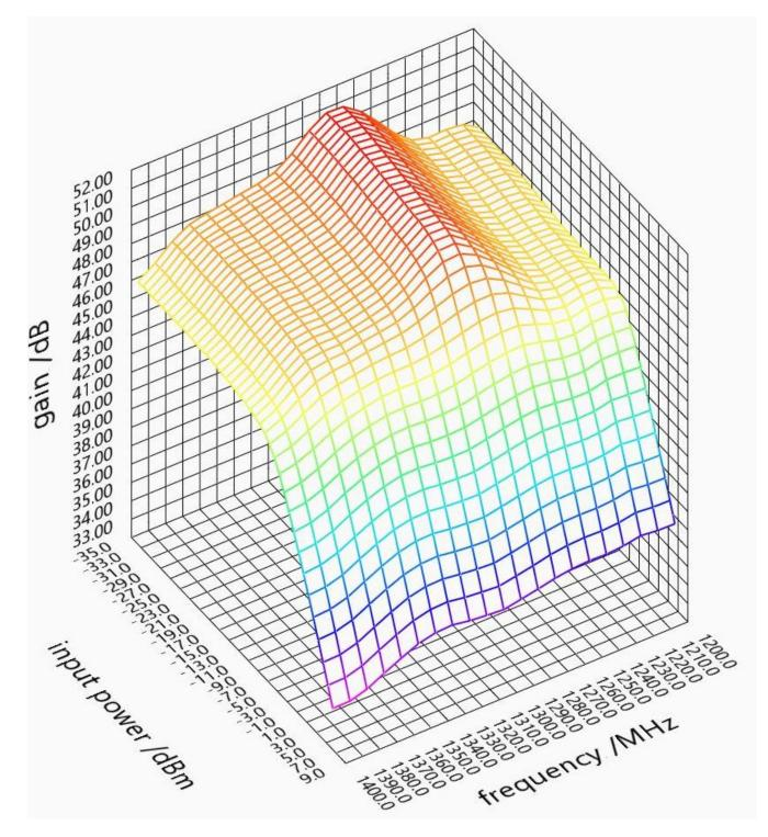
Here is measured gain in dB versus frequency in MHz and input power in dBm.
