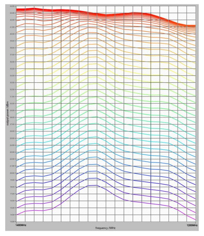
In the next graph you see the measurement of output power as a function of input power (both in dBm). The different curves reflect different frequencies.
