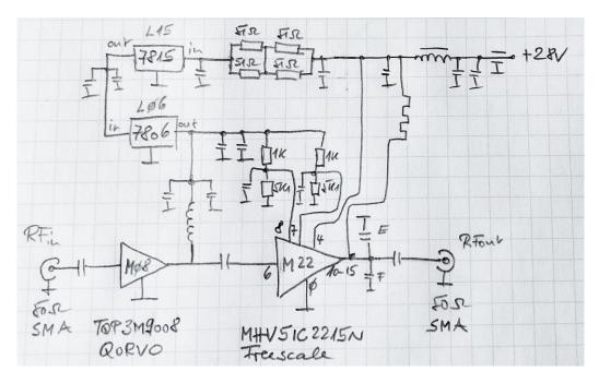
The seller clearly states that the PA modules needs to be mounted on a heatsink. I clamped the module on a heatsink and characterized the driver amplifier using an automated test setup. The used signal generator is a R&S SME03, the power meter is a R&S URVD with a diode test head NRV-Z7.
