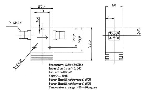
The isolator has female SMA connectors at the input and output port. The internal resistor is attached to a little heatsink. Even though it is specified to handle 50W mode in both directions I am not sure that this can be sustained in CW mode for a longer period of time in case of a complete mismatch at the output.
