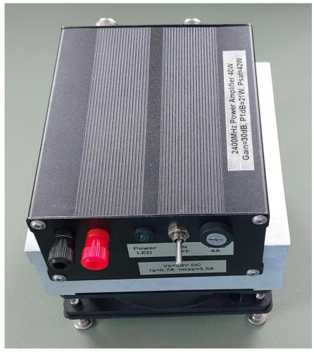
The heatsink is from a flea-market and is adequate for this kind of PA. The stand-offs can be easily removed in case this PA gets integrated together with a 28V power supply in a larger encasing.
