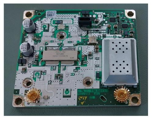
First, I planned to repair the PCB, as the LDMOS transistors themselves seem to be still ok. Then I saw a nice description "Modification the driver stage of SSPA UMTS module to 2320 and 2400 MHz" from Tom SP5XMU and Andrzej SP8XXN and decided to modify the damaged pallet accordingly. Tom and Andrzej were using only the driver stage of the pallet and obtained an output power of 35-42W with an input power of 60mW.
