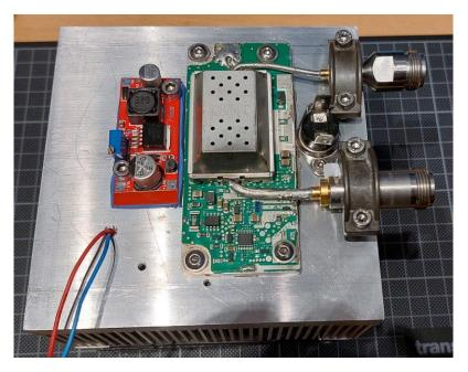
I am using a fan with a supply voltage range 12-24V. Normally it is supplied with 13V (by adding a suitable series resistor) which is perfectly fine for lower output levels and as the fan runs with lower speed it is rather quiet. Once the temperature of the heatsink exceeds 50V, the resistor is bridged by a thermo-switch and the fan runs with full speed at 28V supply voltage. You can see the switch between the RF board and the coaxial connectors.
