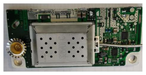
First, I cut off the driver stage from the pallet and then modified the input and output matching circuitry around the driver IC MW7IC2240N according to their excellent description. I will not repeat this modification in my description as I followed exactly their description which you can find here: <a href="http://www.sp5xmu.pl/13cm/MW7IC2240N%20">http://www.sp5xmu.pl/13cm/MW7IC2240N%20</a> 35W new approach.pdf
