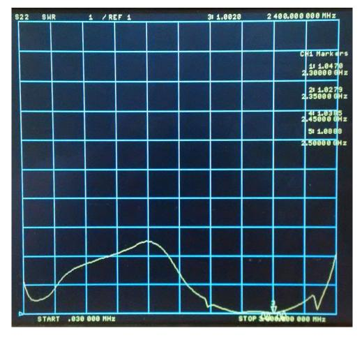
The measurements show that this isolator is very well suited to cover the frequency range 2.3 - 2.5GHz. It is well centered in the 13cm band. At 2400MHz it features an insertion loss of 0.37dB and an excellent isolation of 39.7dB. Input and output return loss are 35dB and 60dB respectively.
