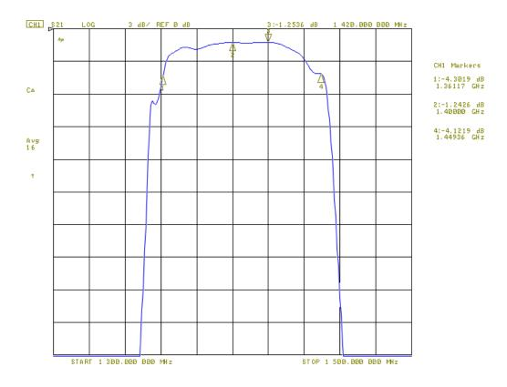
Insertion loss S21 is 1.25dB @1420MHz.
