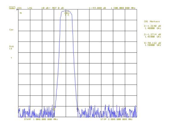
Insertion loss in opposite direction S12 is almost identical to S21.
