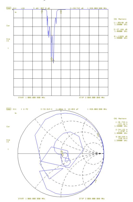
Input return S11 loss is 30dB @1420MHz.
