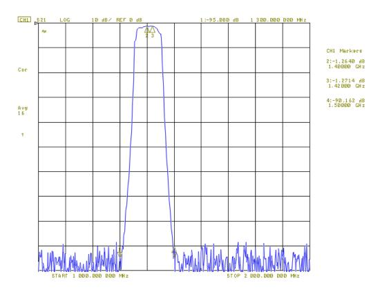
The filter shows an extremely high selectivity with a suppression of more than 90dB of signal below 1300MHz and above 1500MHz.
