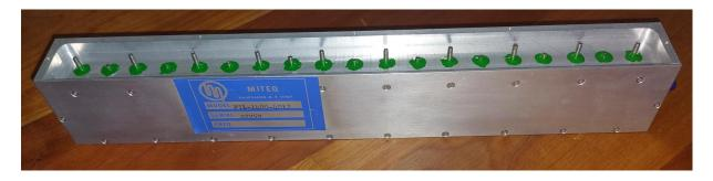
Retuning the filter to 1420MHz worked very resulting in an insertion loss of less than 1.3dB.
