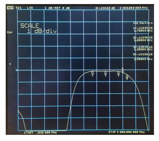
S12 reverse transmission (isolation at 32.4@1700MHz, 26.0@2300MHz, 18.5dB@2400MHz)
