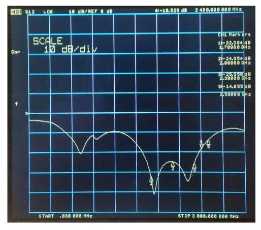
S22 output matching (return loss at 31.4@1700MHz, 27.2dB@2300MHz, 19.4@2400MHz)
