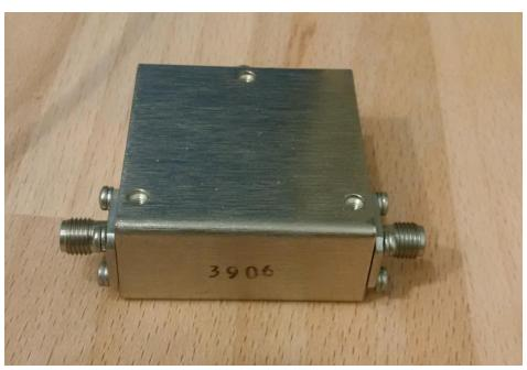
The circulator is in a solid metal case and has 3 female SMA connectors. It has a frequency range 1.7-2.3GHz printed on the label. Below you will find some measurement results of this S-band isolator. All measurements were done in the frequency range 30kHz to 3GHz.
