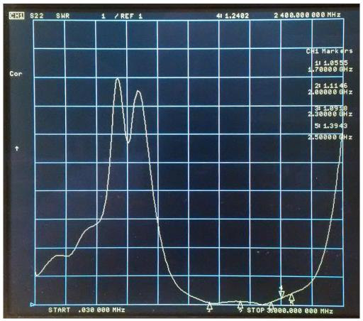
The measurements show that this isolator is very well suited to cover the frequency range 1.7 - 2.3 GHz.
