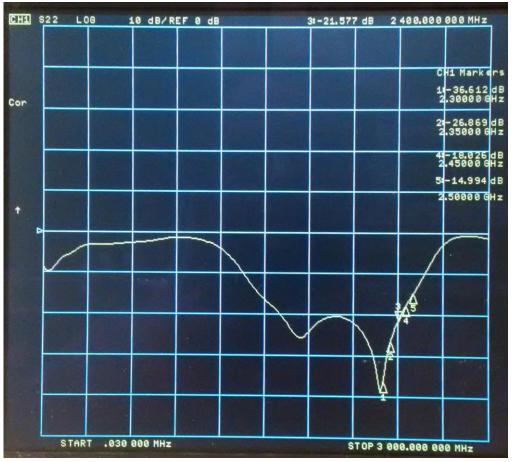
The measurements show that this isolator is well suited to cover the frequency range  $1.7 - 2.4 \, \text{GHz}$ .
