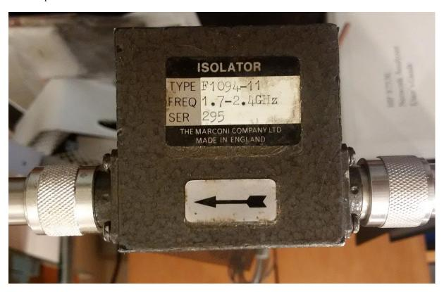
The isolator is in a solid metal case and has female N connectors at the input and output port. It has a frequency range 1.7-2.4GHz printed on the label.
