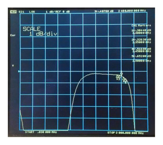
S12 reverse transmission (isolation at 1700MHz is >25dB and at 2400MHz it is -23.7dB)
