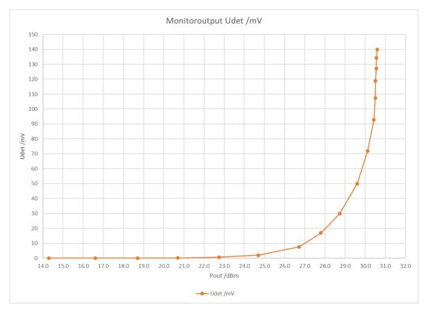
This amplifier module features a directional coupler at its output. The coupler is printed on the PCB and the forward power is measured by a diode detector. Below please find the measured detector voltage versus output power at 2.4GHz. In the first diagram the x-axis is logarithmic (dBm), in the second it is linear (mW).
