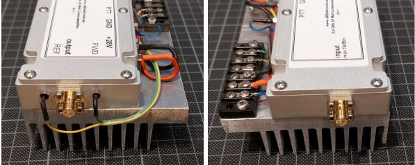
First, I measured output power and gain of the amplifier versus its input power at 2.4GHz using a supply voltage of 28V (internally 27.3V). I also measured the current consumption in order to be able to calculate the efficiency of the complete module as a function of input / output power. During this measurement, the DIP-switches inside the module were set for maximum gain of the amplifier (D0 to D5 were set to 1).
