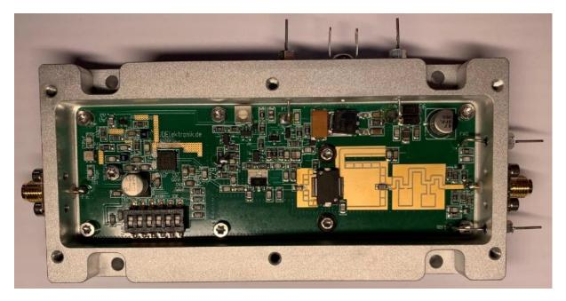
The RF input signal is first passing a SAW filter centered at 2.4GHz and then amplified by a first BGA614 MMIC stage.
