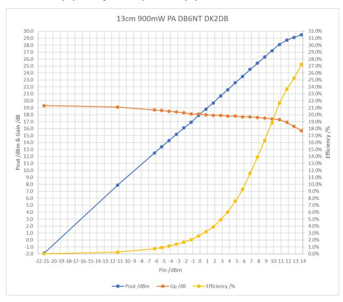
First, I measured output power and gain of the amplifier versus input power at 2.4GHz.
