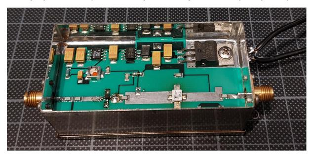
The first stage is based on a MMIC with the marking "E5"; thus, it is most likely an ERA5 from Mini Circuits. The ERA5 MMIC needs a supply voltage of 5V which is generated by dropping the 10V supply voltage by a 680hm resistor. This assumes a current of 74mA which is a bit higher than the typical operating current of 65mA but well within the operating range limits of maximum 85mA. At 2.4GHz the ERA5 should give a typical gain of 18dB at 2.4GHz.
