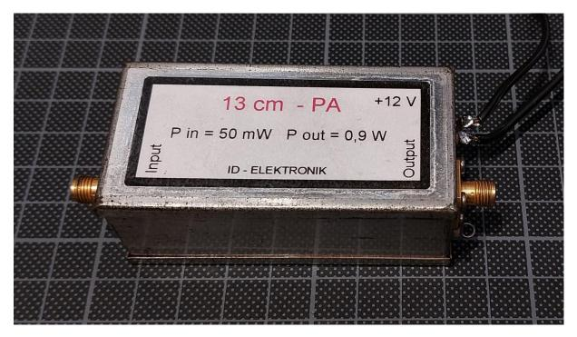
The amplifier is comprised of a high pass filter followed by a two-stage amplifier and a directional coupler with a diode detector (please not the in the picture below the input is right, the output is left).
