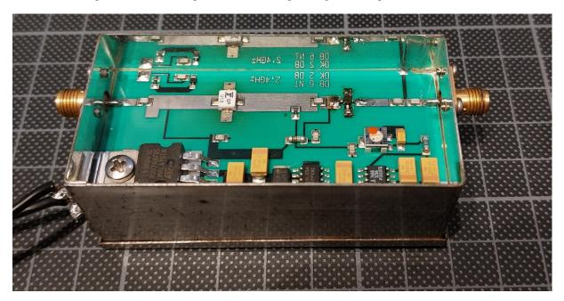
The supply voltage is stabilized to 10V by a L4940V10 low drop voltage regulator from ST Microelectronic. This is also the drain voltage of the second stage. The negative gate voltage for the GaAs FET is generated by a 5V voltage regulator followed by an ICL7660 voltage inverter and a potentiometer to adjust the gate voltage.
