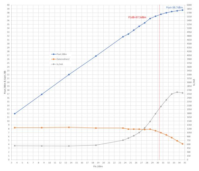
Pout, Gain and Is versus Pin @2400MHz
