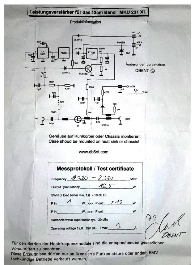
This PA is supposed to give a saturated output power of 12W at a supply voltage of 12V. Here is a description of the PA probably given by the supplier with that unit when it was shipped:
