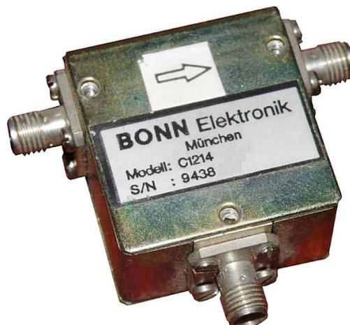
This is a picture of the isolator (already hooked up for the measurements):
