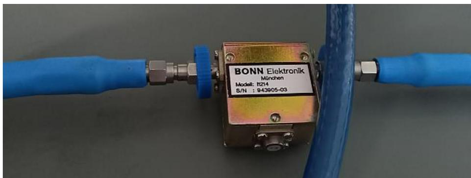
As I needed an isolator for a 23cm power amplifier which I am presently building I measured one of the isolators. I performed measurements of the S-parameters in the frequency range 1000 – 1500 MHz.
