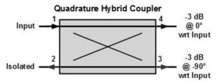
Sometime last year I got a PCB with an etched branch-line coupler from DD1IA. He had bought it from PE1RKI but never tested it himself. The coupler should work at 2.4 GHz and handle up to 2 times 100W input power as a combiner.
