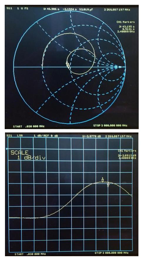
S21 log mag at 2267 MHz is -2.88dB. S21 log mag at 2400 MHz is -2.89dB.
