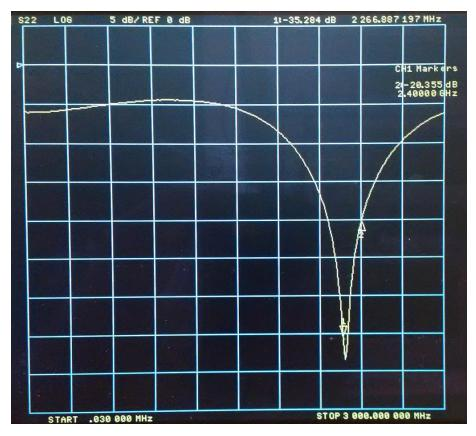
S22 log mag at 2267 MHz is -35dB. S22 log mag at 2400 MHz is -20dB.
