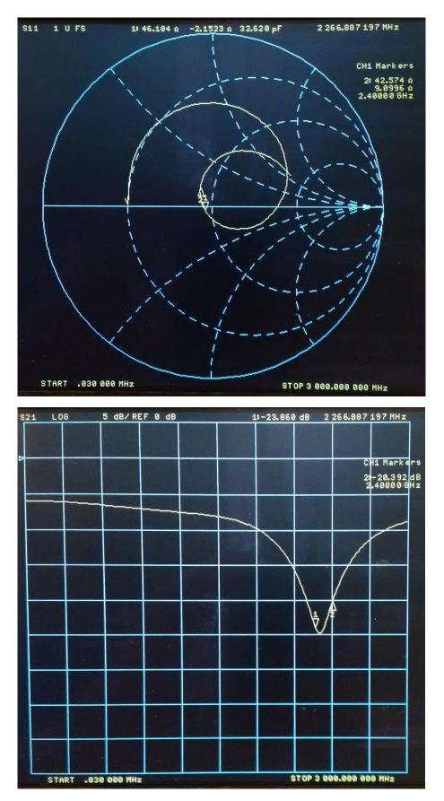
S21 log mag at 2267 MHz is -23.9dB. S21 log mag at 2400 MHz is -20.4dB.
