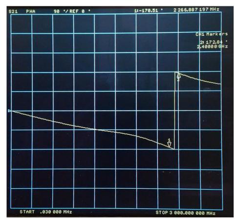
S21 phase at 2267 MHz is 170.51 degree, at 2400 MHz it is 172.84 degree.
