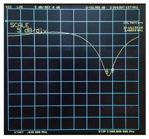
S22 log mag at 2267 MHz is -22dB. S22 log mag at 2400 MHz is -19dB.
