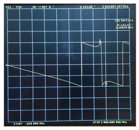
S21 phase at 2267 MHz is 161.9 degree, at 2400 MHz it is -141.6 degree.
