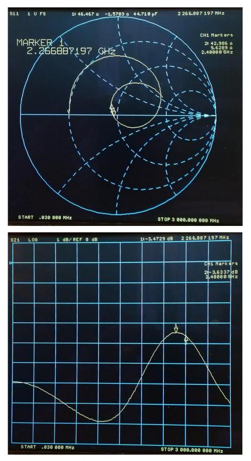
S21 log mag at 2267 MHz is -3.47dB. S21 log mag at 2400 MHz is -3.64dB.
