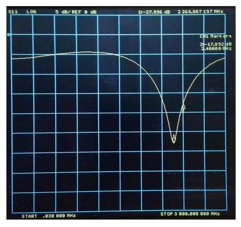
The quadrature coupler is rather narrowband and shows a clear resonance frequency at 2267 MHz. Input return loss S11 is -28dB. At 2400MHz the return loss S11 is only -18dB.
