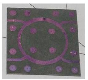
I cleaned the Teflon PCB and silver plated it. Then I mounted it on a surplus brass plate (which is gold plated which makes it look like  $\bigcirc$ ) in order to be able to test it.
