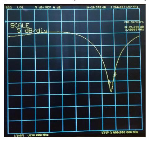
S22 log mag at 2267 MHz is -27dB. S22 log mag at 2400 MHz is -21dB.
