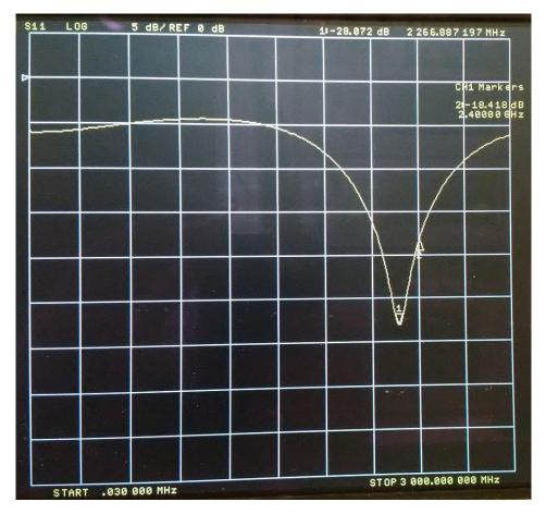
Input return loss S11 at 2267 MHz is -28dB. At 2400MHz the return loss S11 is only -18dB.
