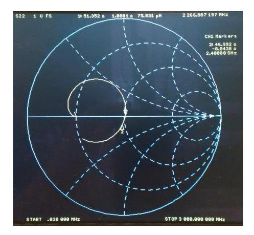
This is the summary of the parameters of the hybrid coupler measured at 2267 MHz:
