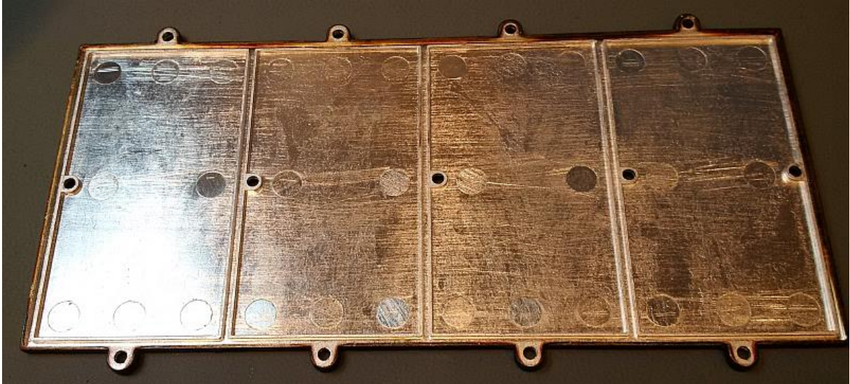
After splitting the 2 parts of the duplexer I assembled 2 SMA jacks on each of the open parts.
