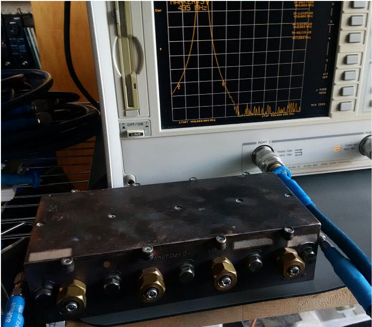
After splitting the 2 parts of the duplexer I assembled 2 SMA jacks on each of the open parts.
