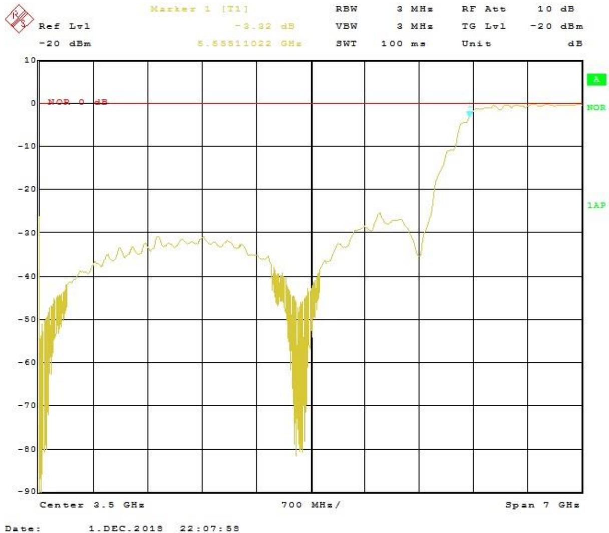
As you can see the 3dB cutoff frequency is at approximately 5.55 GHz and also the complete curve fits quite well with the reference plot in the datasheet. Also, the insertion loss is in spec.
