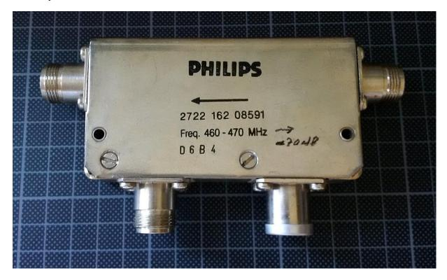
Below you will find some measurement results of this circulator for the 70cm band. In the first series of measurements the  $3^{rd}$  port was terminated with 50 Ohms.
