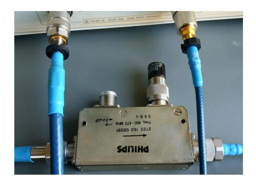
S11 input matching (return loss 33dB@430 MHz, 50dB@440MHz)
