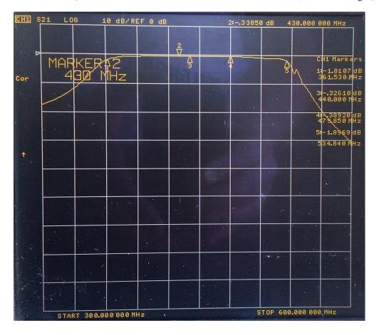
S12 reverse transmission (isolation is 32dB@430MHz and 37dB@440MHz, much reduced due to the open port)
