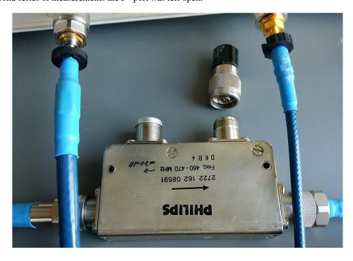
S11 input matching (return loss 33dB@430 MHz, 50dB@440MHz, same as with termination of port 3)
