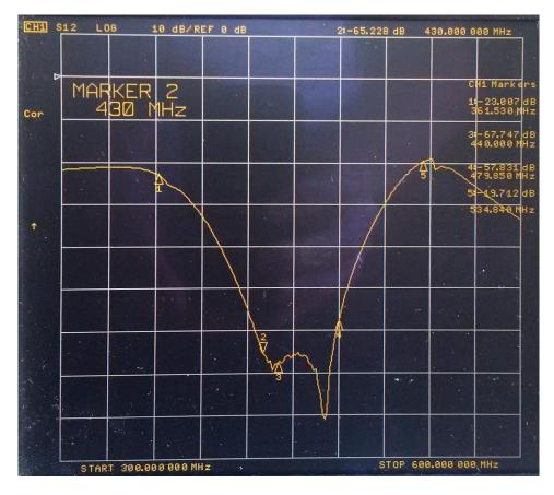
S22 output matching (return loss is 28.5dB@430MHz and 440MHz)
