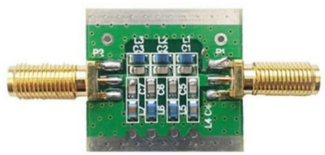
The band reject filter is comprised of 4x LC series resonance and 3x LC parallel resonance sections.
