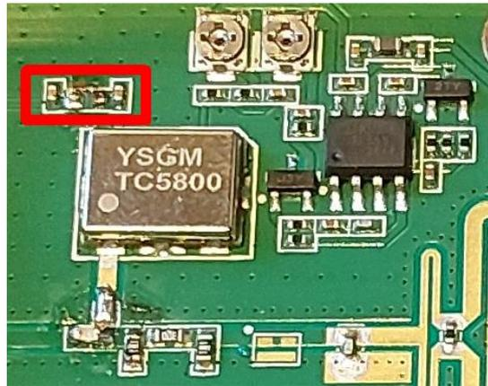
The quiescent current of the PA was originally set to approx. 2.2A. I found that setting a quiescent current of 0.7A resulted in the same maximum output power and a more linear gain versus input power without excessive gain peaking around the P1dB. The quiescent current can be set b with a small trimmer on the board:
