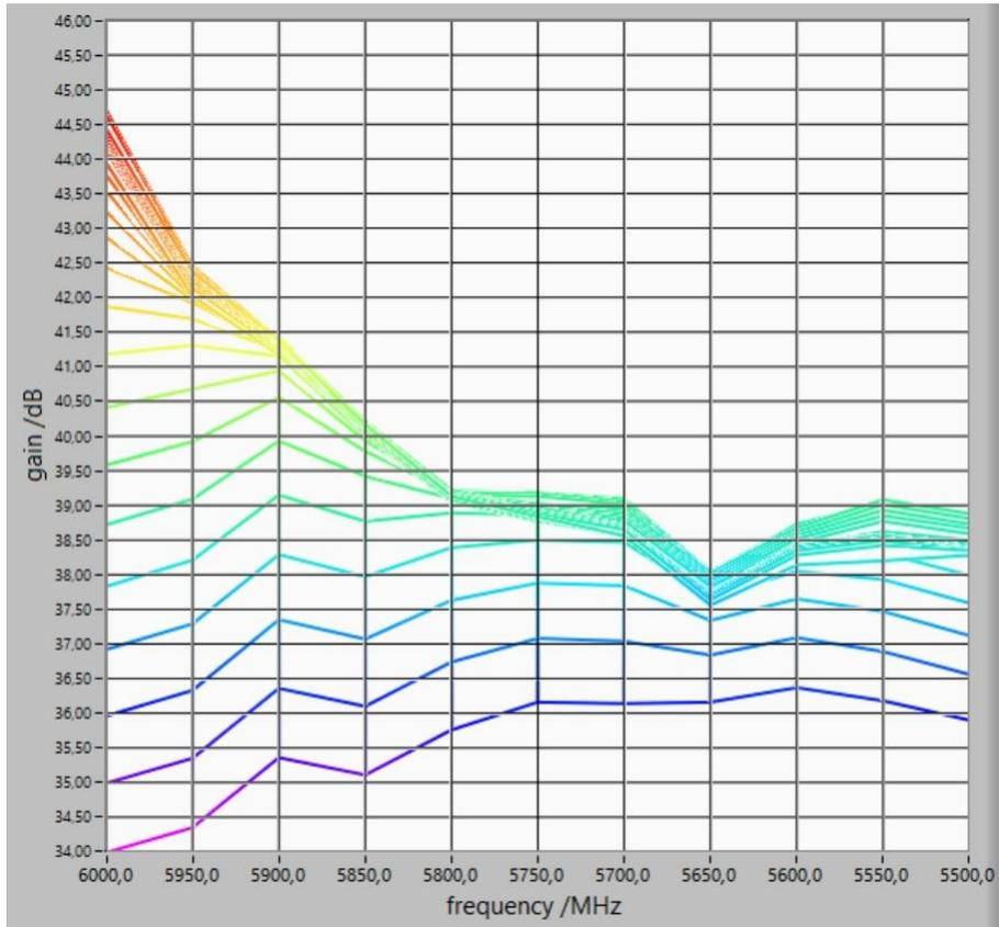
Gain /dB as a function of frequency /MHz and input power /dBm
