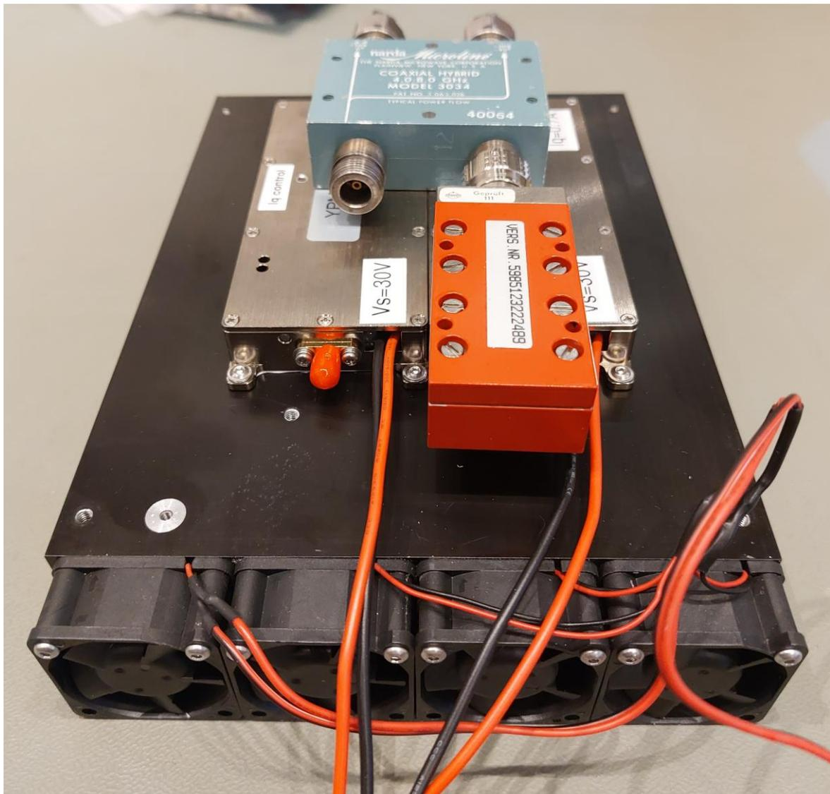
The short jumper connections from SMA male to N-male turned out to be not good for 5700MHz. I assume it is due to the right angle N-connectors and I replaced them with straight connections. The isolation port of the output combiner is terminated by a Spinner BN-527711 50Ohm dummy load with a maximum power of 25W. If needed it can be mounted on a heatsink which will increase the maximum power to 80W. This dummy load turned out to have an excellent return loss at 5.7GHz of more than 30dB.
