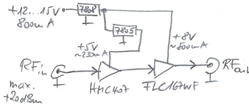
In order to be able to use the 12V power supply I added a second voltage regulator reducing the voltage from 12V to 8V. Here are the measured parameters of the modified amplifier:
