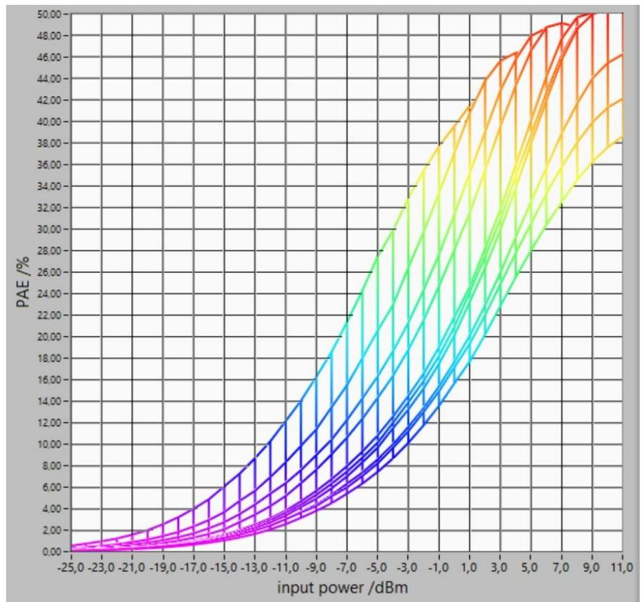
Power added efficiency % as a function of input power /dBm
