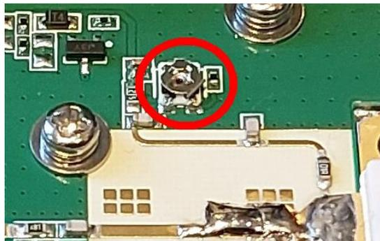
In addition, I slightly tuned the output match of the final transistor for optimum output power and efficiency. This resulted in a slight improvement of output power (ca. +0.2dB) and efficiency (ca. +5%). I tuned some more modules and the tuning was slightly different for each module. Even without tuning the modules works quite well.
