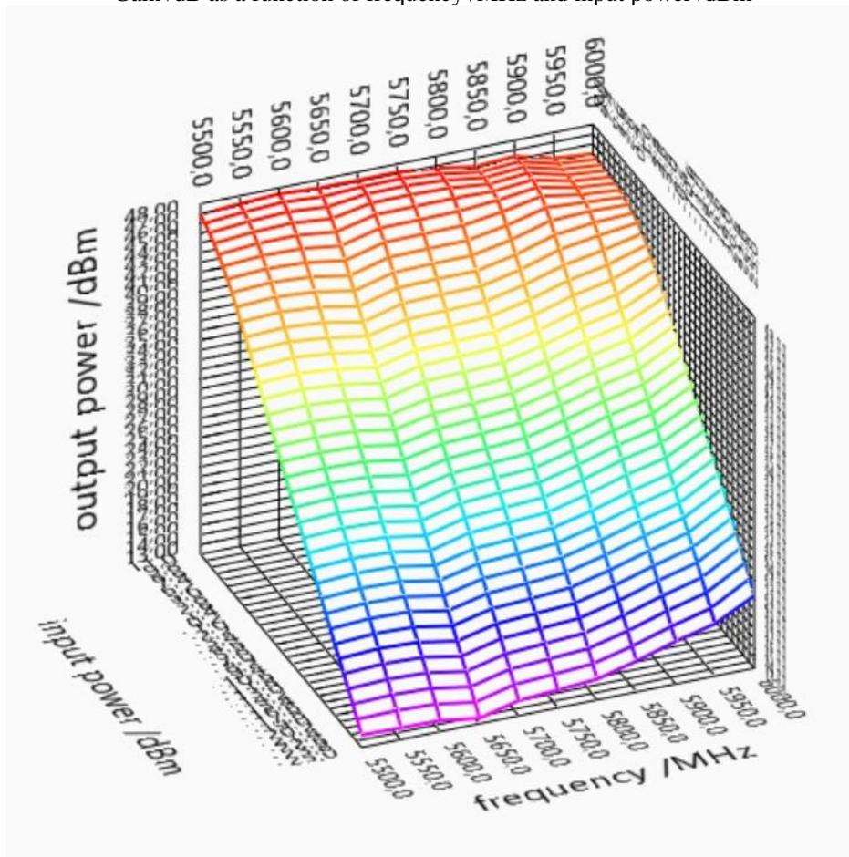
Output power /dBm as a function of frequency /MHz and input power /dBm
