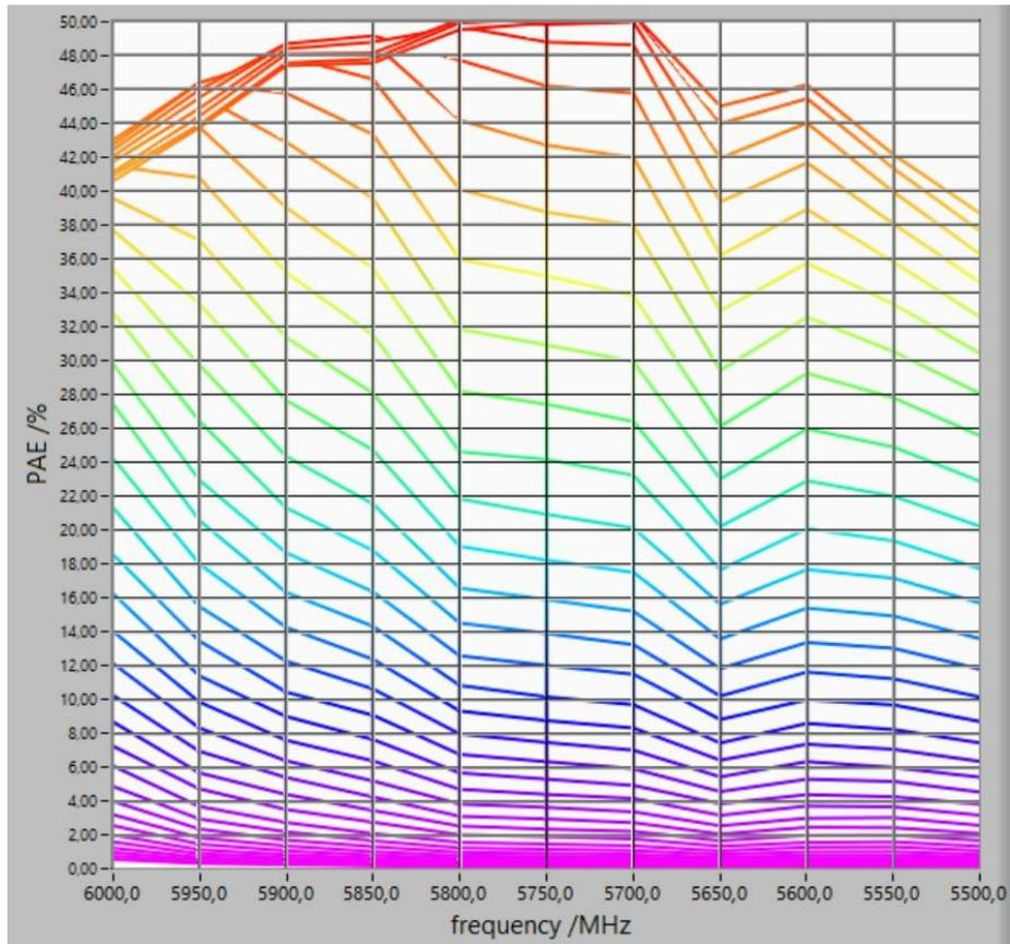
Power added efficiency /% as a function of frequency /MHz
