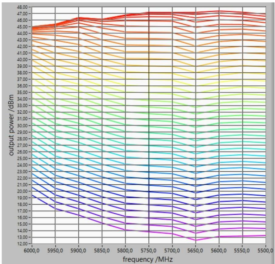
Output power /dBm as a function of frequency /MHz
