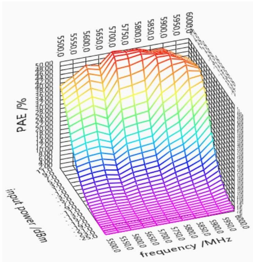
Power added efficiency /% as a function of frequency /MHz and input power /dBm
