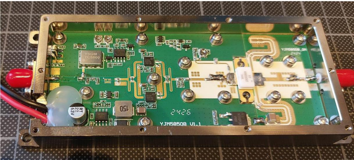
Each SiGe SE5003L MMIC is operated with a single supply voltage of +5V and provides a gain of 32dB and maximum output power of +23dBm. The current consumption is typically 340mA.
