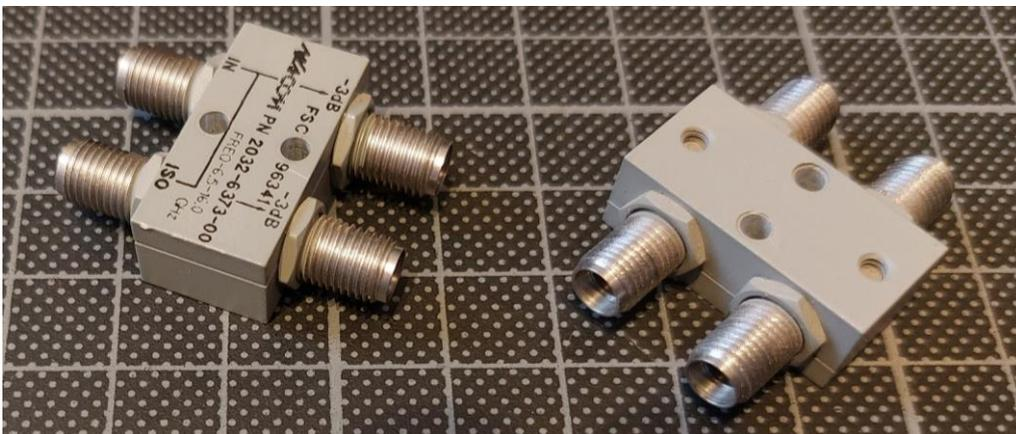
Over the full frequency range this coupler is specified to have a maximum amplitude imbalance of  $\pm 0.5\text{dB}$ , maximum insertion loss of 0.5dB and a minimum isolation of 18dB. The maximum VSWR at all ports is 1.35 which corresponds to a return loss of 16.5dB. It can handle a maximum continuous power of 30W.
