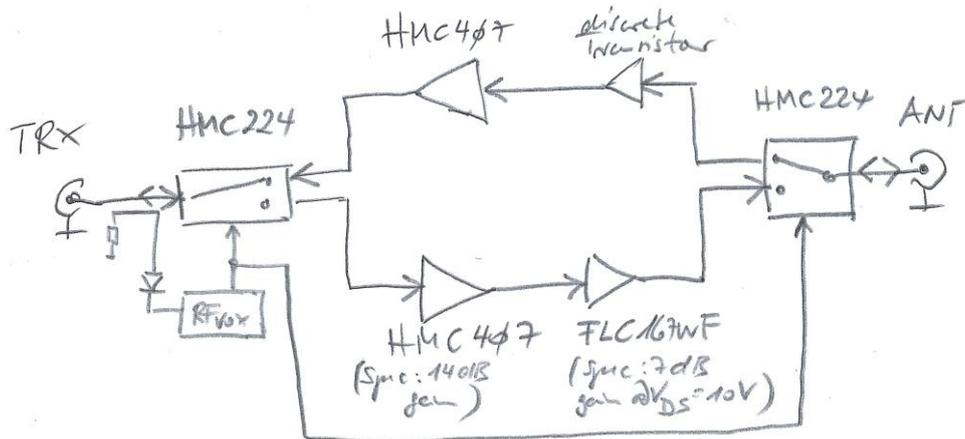
This modules provided a TX gain of 14dB and a RX gain of 17dB, The measured maximum output power was 24.65dBm with an input power of 11.4dBm.
