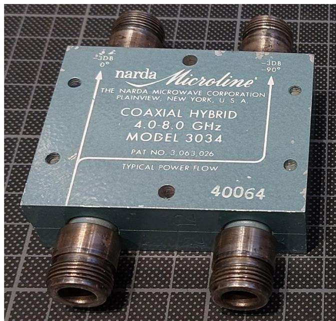
I measured the performance of the coupler at 5.75GHz (port numbering clockwise with In=port1, -3dB/0°=port2, -3dB/-90°=port3, ISO=port4):
