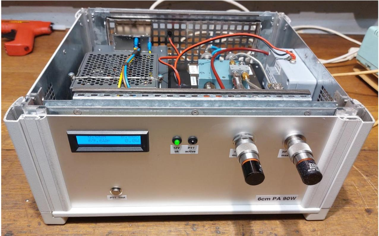
I mounted a DC voltage and current meter for the 30V power supply and two LEDs as indicators for the 12V voltage (green) and the activated PTT (blue) in the front plate. In addition, I added a push button switch to be able to activate the PTT / switch the PA module on for testing.
