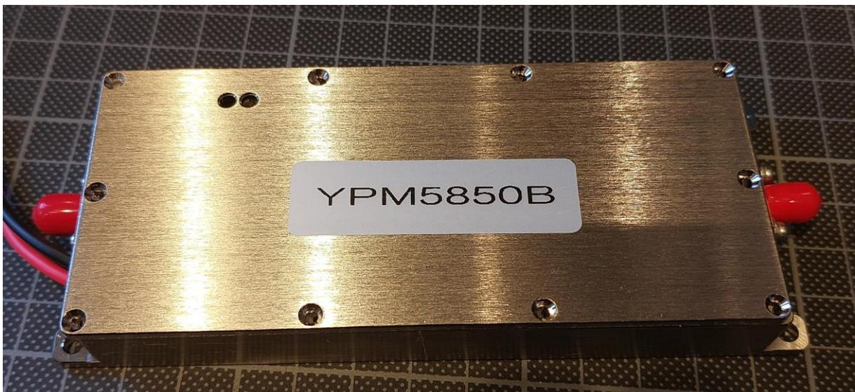
The PA is housed in a compact aluminium encasing and is a two-stage amplifier with the first stage comprised of two MMIC amplifiers SiGe SE5003L operating in parallel and the second stage based on a GaN HEMT transistor with the part number YP40601650T from Innotion. Here are some pictures of the opened PA module:
