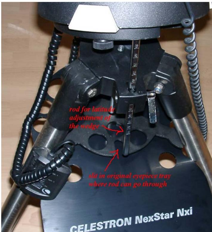
One additional hole has to be drilled in the tray for the latitude adjuster
