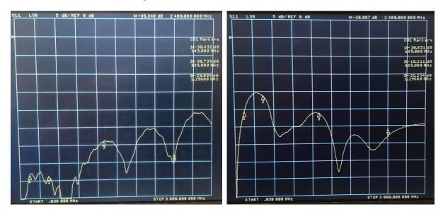
The minimum return loss observed at different setting was 15dB. S22 is basically identical to S11.
