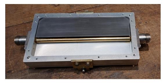
We can see the gold-plated center conductor and above a U-shaped black block of unknow material. I suppose it is made from a ferrite material.
