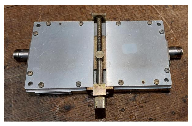
Input and output ports are N-jacks. Turning the screw on the bottom of the picture will move the vertical adjustment slide up and down.
