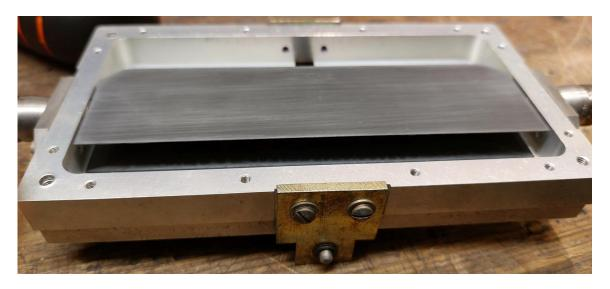
When the U-shaped block is completed moved up / not covering the centre conductor the minimum insertion loss is achieved. The further the block is moved over the centre pin, the higher the insertion loss. In the next picture you see the position of the block when maximum insertion loss is achieved:
