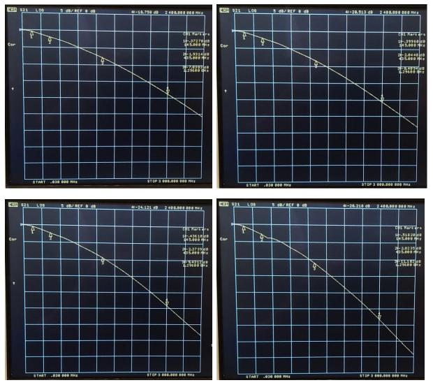
As can be seen the insertion loss is highly frequency dependent. At low frequencies the change of attenuation is very low. The minimum insertion loss is 0.03dB @145Mhz and 1.53dB @2.4GHz. The maximum attenuation is 0.52dB @145MHz respectively 28.22dB @2.4GHz. Measured S12 is bascially identical to S21.
