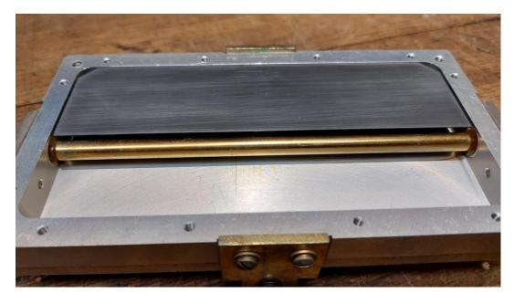
When turning the before mentioned screw the vertical adjustment slide will move that U-shaped block up and down (moving over the centre conductor without touching it).
