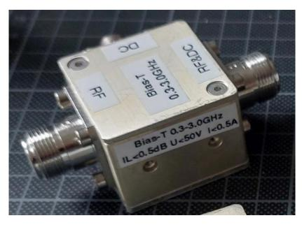
Next, I built the Bias-T with BNC connectors. I had to shorten the PCB and make compromises with respect to the connection of the ground plane of the PCB to the encasing. You can see that the frequency response of the insertion loss is almost identical at lower frequencies but the maximum frequency range is limited to about 2.5GHz certainly due to the less optimum ground plane connection.
