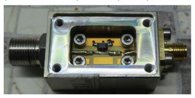
I used a broadband conical inductor from Coilcraft with an inductivity of 1.65uH (BCL-162JL) and a maximum current of 490mA. They are optimized for ultra broadband Bias-Ts as can be seen in the specifications below (data from Coilcraft measured in a Bias-T setup).
