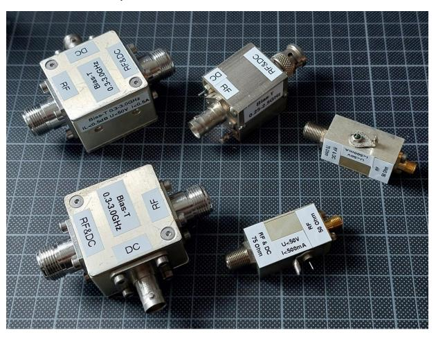
I started with the encasings featuring N-jacks at input and output. Originally also the 3<sup>rd</sup> port was using an N-jack but I replaced it with a BNC-jack as this port will be used to inject the DC supply. The PCBs fit perfectly in the surplus encasings.
