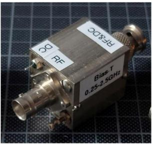
Finally, I modified the  $50\Omega$  to  $75\Omega$  impedance transverter modules. The are very well built in a solid milled aluminium encasing. The impedance conversion is accomplished using a transformer. The PCB provides enough space to add the needed inductor and two capacitors to block the DC port from the RF path.
