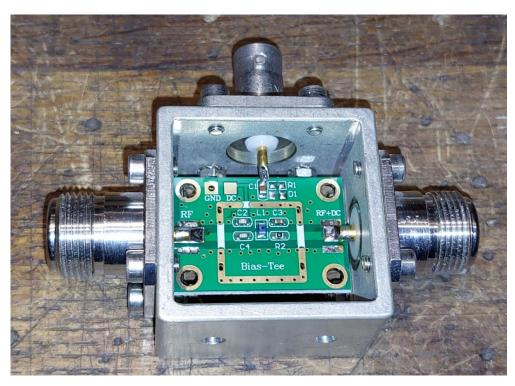
Special care was taking to provide a good ground connection to the PCB.
