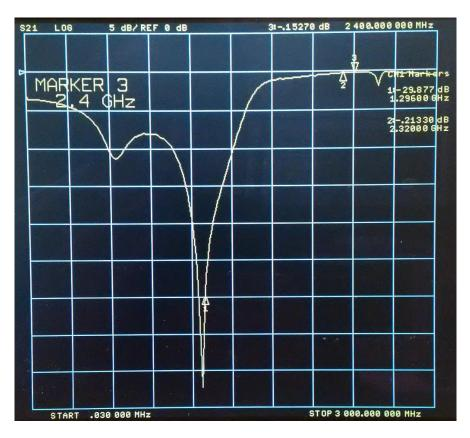
Insertion loss S12 from the 13cm port to the common port is basically identical to S21.
