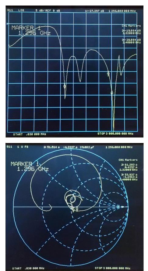
Insertion loss S21 from the common port to the 23cm port is 0.20dB at 1296 MHz. Stop-band attenuation at 2320 MHz is 26.9dB and 52dB at 2400 MHz.
