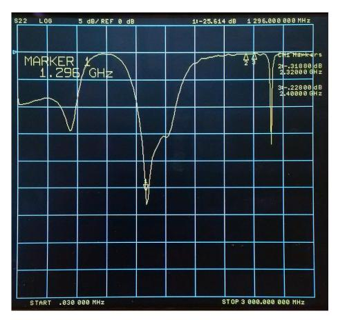
In the next series of measurements, I used the common port as port #1 and the 13cm port as port #2. The 23cm port was terminated with 50 Ohms.
