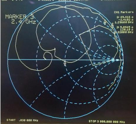
In the next series of measurements, I used the common port as port #1 and the 13cm port as port #2. The 23cm port was terminated with 50 Ohms.
