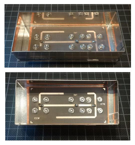
After performing my first series of measurements I had to notice, that stop band attenuation at 13cm, when measuring S21 from the common port to the 23cm port, was only 14dB. In addition, insertion loss at 13cm, when measuring S21 from the common port to the 13cm port, was almost 1dB. Therefore, I optimized the setup including tuning some open stubs by cutting them with a scalpel. Here is a picture of the same unit after the optimization:
