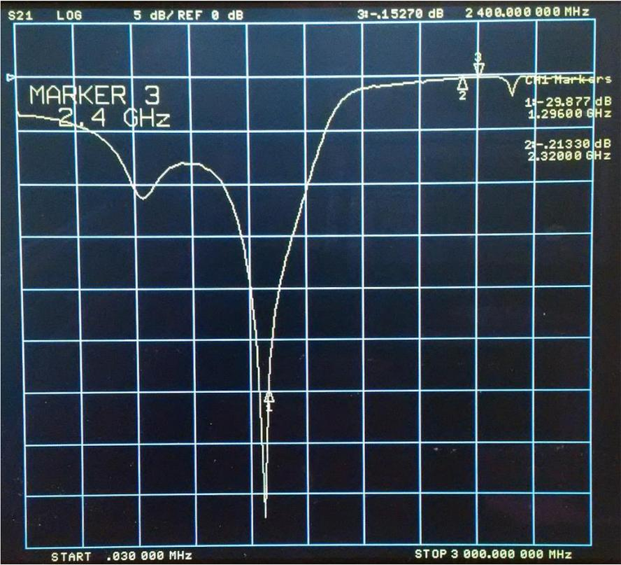
Insertion loss S12 from the 13cm port to the common port is basically identical to S21.
