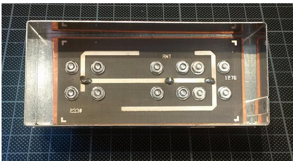
After performing my first series of measurements I had to notice, that stop band attenuation at 13cm, when measuring  $S_{21}$  from the common port to the 23cm port, was only 14dB. In addition, insertion loss at 13cm, when measuring  $S_{21}$  from the common port to the 13cm port, was almost 1dB. Therefore, I optimized the setup including tuning some open stubs by cutting them with a scalpel. Here is a picture of the same unit after the optimization:
