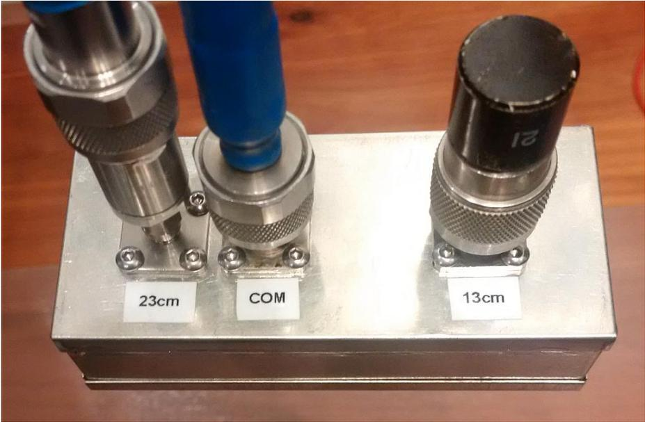
Input matching S11 of the common port is 26dB at 1296 MHz and 14.3dB at 2400 MHz.
