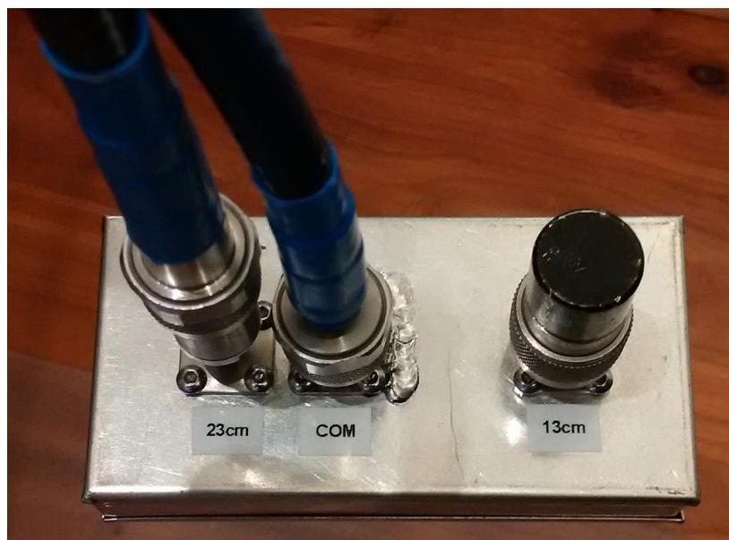
Input matching S11 of the common port is 27.3dB at 1296 MHz and 28dB at 2400 MHz.
