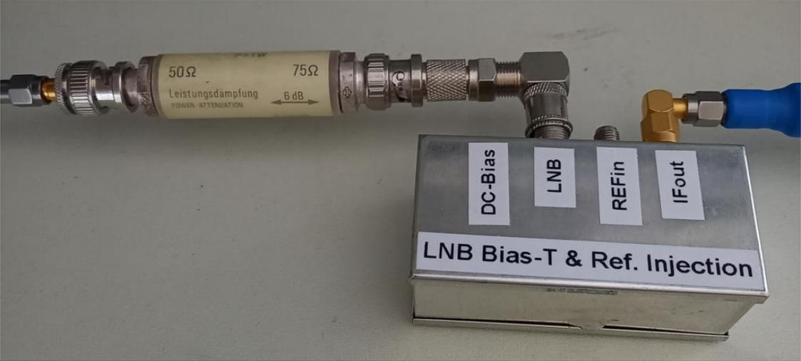
The input matching pad from 75 Ohm to 50 Ohm consisting of R7 and R8 is introducing a nominal loss of 6.1 dB. The PI-attenuator consisting of R1, R3 and R5 has a nominal loss of 10.1 dB.
