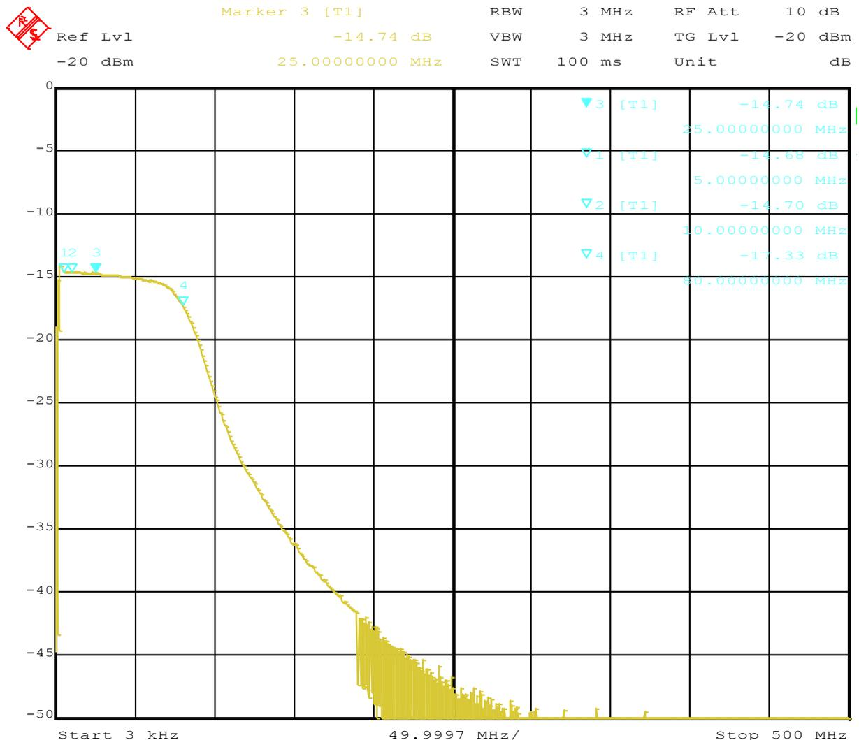
The low pass filter consisting of L1, C2 and L3 has a 3dB cutoff frequency of about 80 MHz and rejects and IF signals coming from the LNB port adequately.
