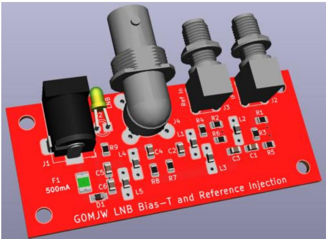
The idea is to “phantom feed” a reference frequency signal of 10, 25 or 27 MHz and 12 to 18 V DC to the LNB and get back the IF signal, all on one cable. At the LNB end one filters off the reference signal and uses it to lock the PLL in the LNB and powers the LNB with the DC supply. Here is the schematic of the module. I have assembled both optional attenuators, which introduce an additional attenuation of 10dB in the LNB-to-IFout path and 3dB in the REFin-to-LNB path.
