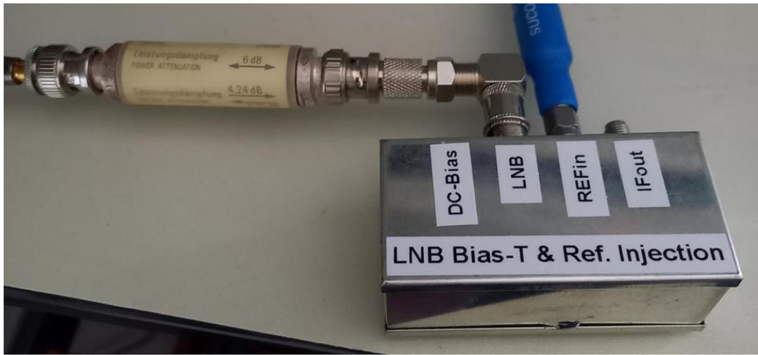
The input matching pad from 75 Ohm to 50 Ohm consisting of R7 and R8 is introducing a nominal loss of 6.1 dB. The PI-attenuator consisting of R2, R4 and R2 has a nominal loss of 3.0 dB.
