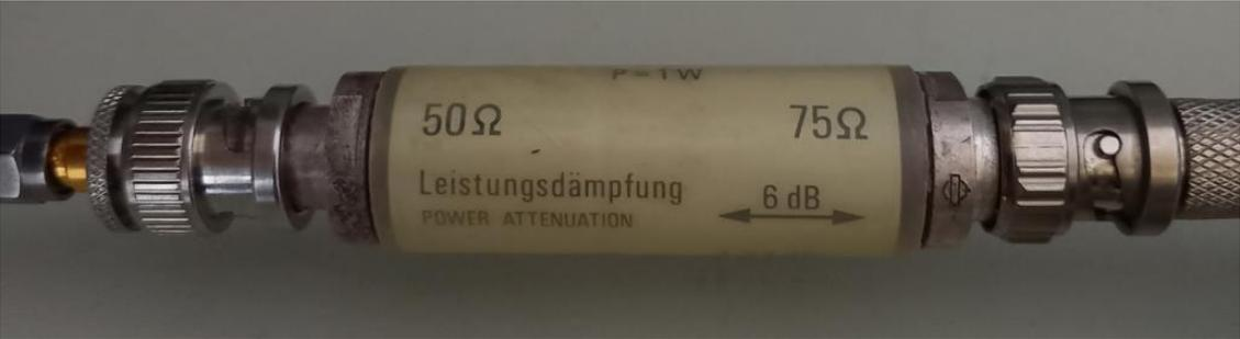
This matching pad provides proper impedance matches but also introduces an insertion loss of 6dB. Thus, the measurements below have to be corrected by 6dB (you can find this in the columns “corrected”).
