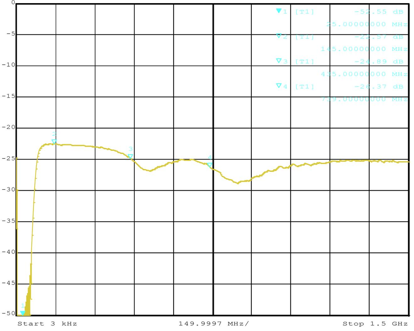
Next, I measured the path from LNBinput to REFin.
