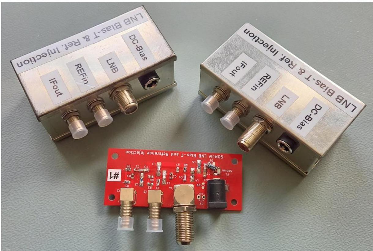
Finally, I found the time to characterize the board. As the LNB port is matched to 75 Ohms and my measurement setup is all 50 Ohms I used a 50 Ohm – 75 Ohm matching pad:
