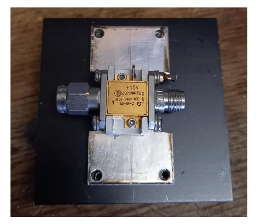
In the picture above the metal cover is missing which helps to clamp the amplifier to the main heatsink below. The clamp itself also acts as an additional heatsink.
