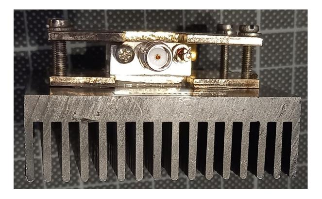
First, I measured gain (blue) and noise figure (red) of the device in the range from 200 MHz up to 18 GHz at the nominal supply voltage of 15 V. The current consumption was 66 mA.
