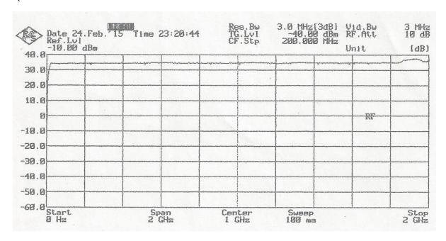
As can be seen the gain is very flat between about 30 and 2000 MHz with approximately 35 dB.
