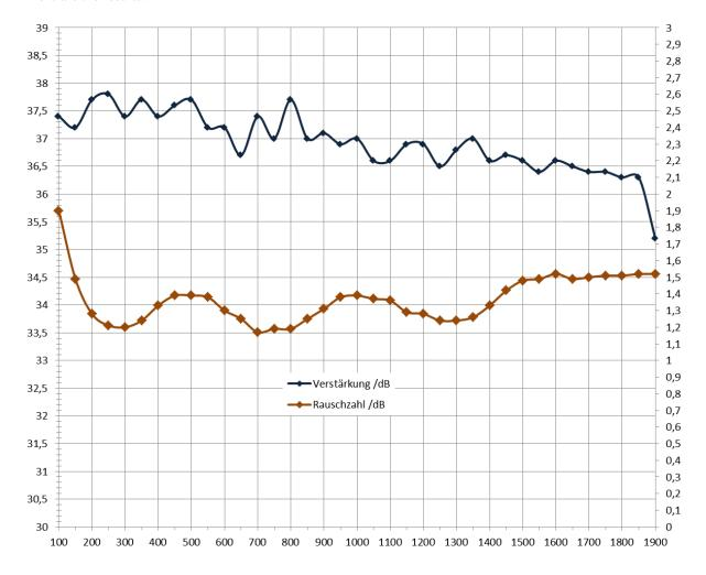
You can see that the gain (dark blue curve "Verstärkung" with the left scale) is quite constantly about 37dB in the range from 100 up to 1900 MHz and the noise figure (brown curve "Rauschzahl" with the right scale) at the same frequency range is about 1.2 to 1.5 dB.
