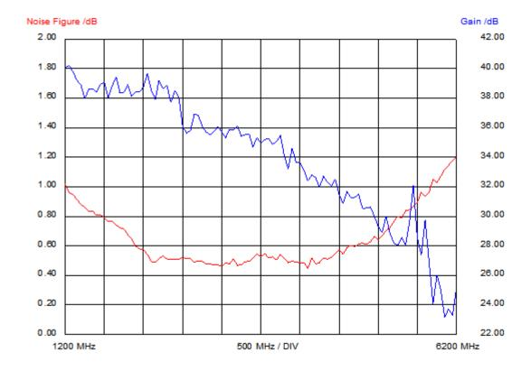
The gain in the range 1200 - 1900 MHz is quite the same as of the first unit. The noise figure of the second unit is a bit lower and interestingly the minimum noise figure of around 0.5dB is achieved in the frequency range 2000 - 4500 MHz. Thus, this amplifier is very well suited as a S-band LNA.
