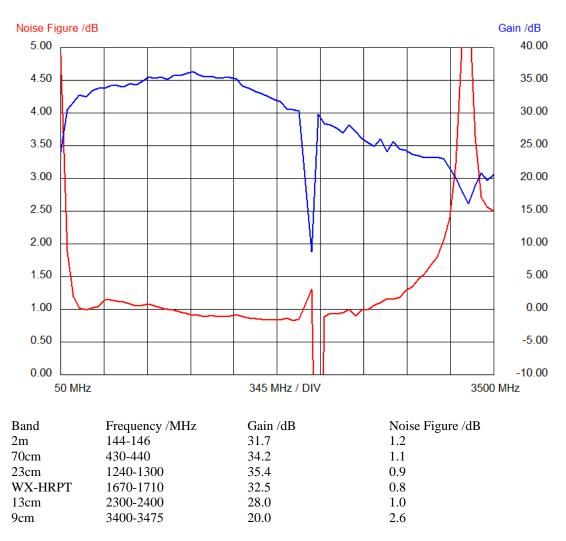
In 2023 I was able to buy another amplifier of the same type. Below please find the measurement results for the second device operated at a supply voltage of 15V.
