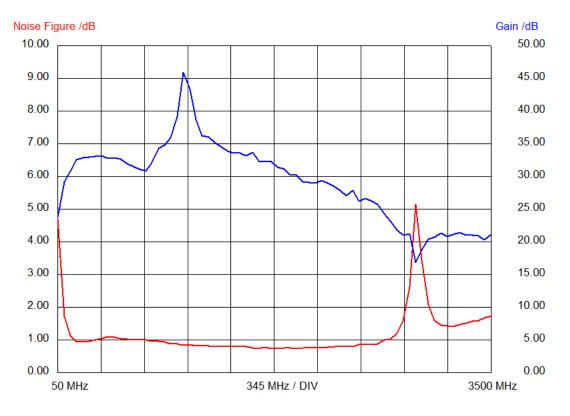
The graph for gain and noise figure are almost the same with gain being about 1dB higher at frequencies below 2 GHz and the noise figure being about 0.1dB better. Here are the respective values:
