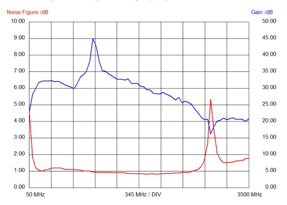
The frequency response of the gain of this amplifier is not really flat. It is around  $32dB \pm 2.5dB$  in the frequency range 150 MHz to 2000 MHz with a strong increase up to 45dB in the range between 950 MHz and 1250MHz. In the frequency range around 2.9 GHz the gain drops down to about 16dB and noise figure rises to more than 5dB.
