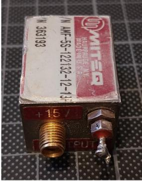
There us a label with the nominal supply voltage of +15V. I measured a current consumption of 138mA.
