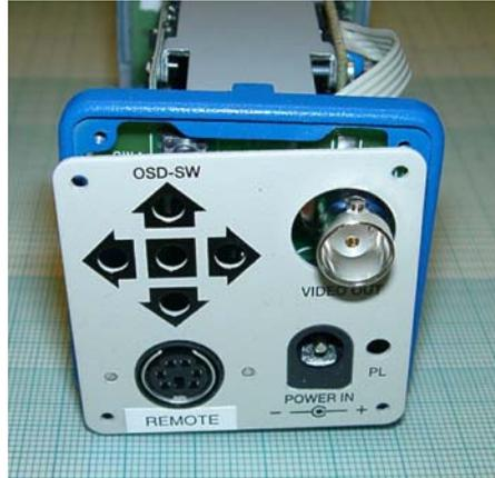
Here the S-Video connector is already replaced by the new 6 pin remote control connector
