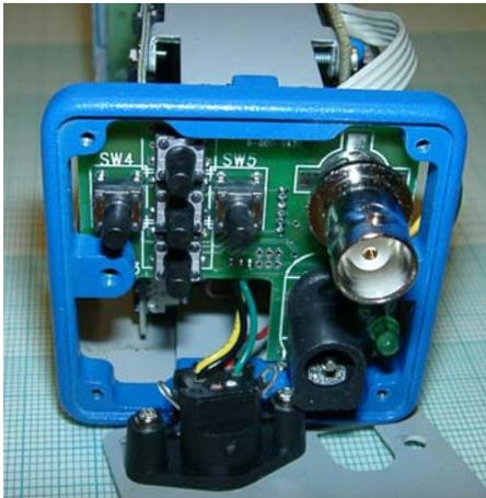
This shows the new remote control connector from the rear
