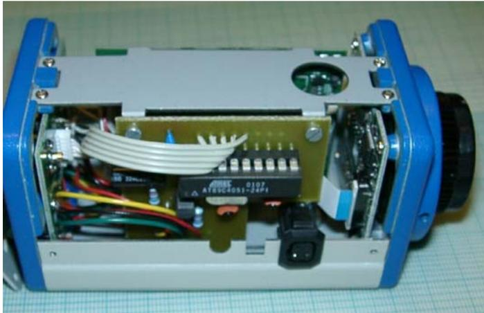
New PCB with ATMEL controller assembled
