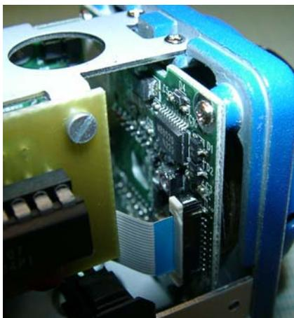
Detail view how PCB is fixed to the existing frame
