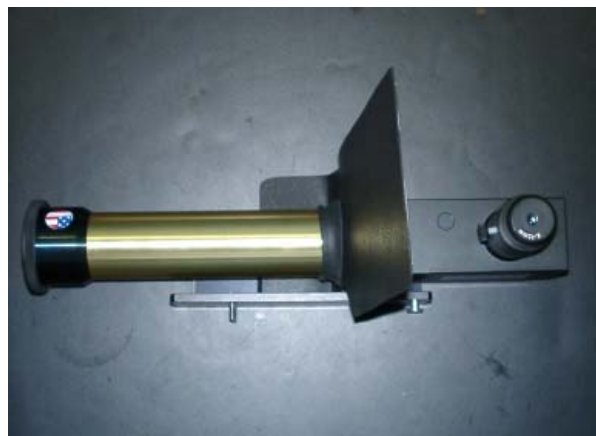
PST mounted on Ray's bracket to attach it easily to an N5i mount, the sun shield is homebrew
