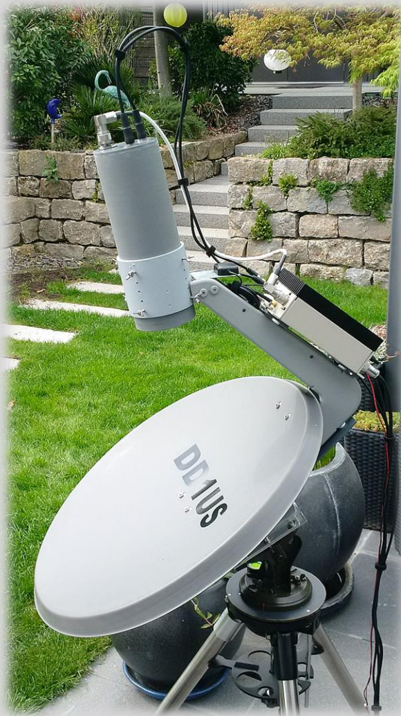
60cm Kathrein offsetdish with AMSAT-DL transverter on feedarm
