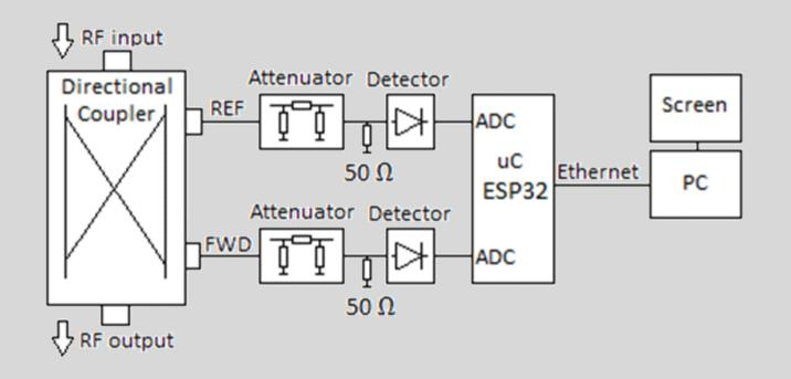
The RF signals decoupled from the directional coupler are passed via attenuators to detectors. These convert the RF signals for forward FWD and reflected REF into DC voltages, which are then digitised by means of AD converters (ADCs).
