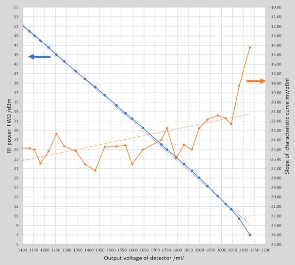
Example of the characteristic curve of the setup measured at 145 MHz. The maximum power of 50 dBm (100 W) was limited by the output power of the transmitter used.
