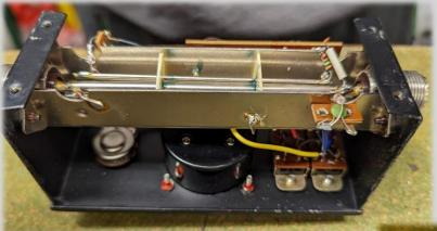
Directional coupler from HF-SWR-Meter Integrated diode detectors
