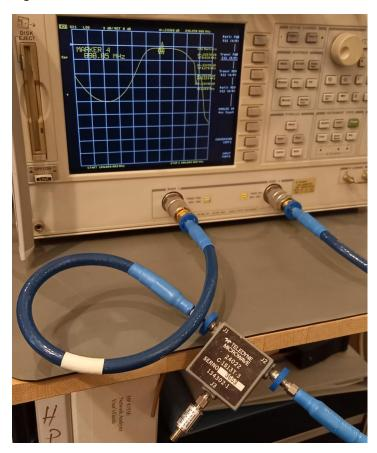
Below please find the measurement results of the S-parameters in the frequency range 100 - 1400 MHz. As all 3 ports show an almost identical behaviour, I will present here only the measurement results from port J1 to J2.
