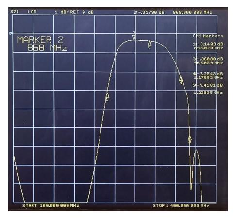
The center frequency of the transfer curve S21 from port J1 to J2 is approximately f=900MHz. The insertion loss at 868MHz is IL=0.32dB. This is excellent.
