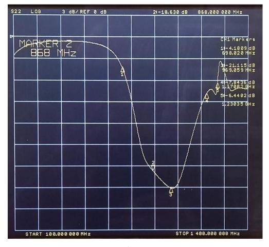
The maximum return loss at port J2 is achieved at f=969MHz with S22=21.2dB. At 868MHz I measured a return loss of S22=18.6dB. The S22 curve and the measured values are very similar to S11.
