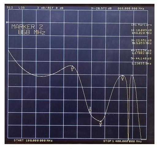
The maximum isolation S12=23dB is reached at f=969MHz. At 868MHz the isolation is S12=21dB, which is good enough for my application.
