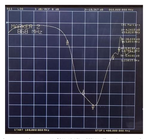
The isolator shows a return loss at port J1 of S11=18.4dB at 868MHz. The optimum return loss is at 969MHz with S11=20.9dB.
