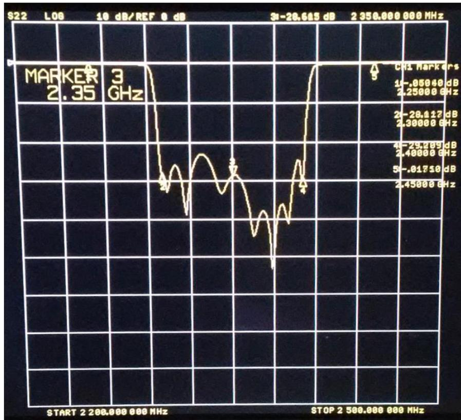
As I want to use this filter primarily to filter my TX signal for the QO-100 narrowband and wideband transponder uplink, I decided to retune it. Before retuning, the insertion loss in the frequency range of the wideband transponder was too high. My target was to reduce the insertion loss in the frequency range 2400-2410 MHz and still keep the nice selectivity of this filter. I found some measurement results published by Manfred DK5FA which showed very promising results.
