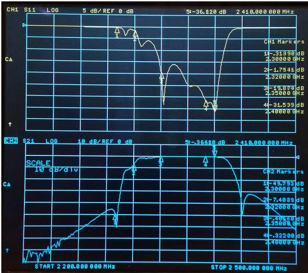
When tuning the filter it is very helpful to monitor both S11 and S21 simultaneously.
