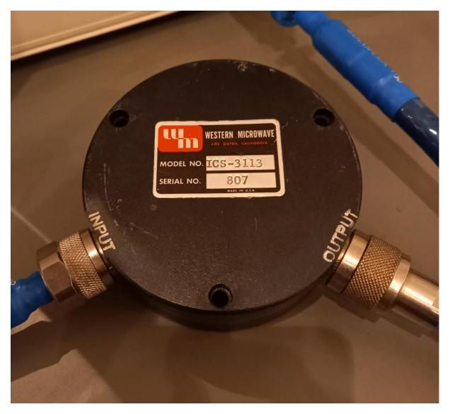
The isolator is in a round plastic case and has female N connectors at the input and output port. There is no indication with respect to the frequency range of the device. The model number is ICS-3113.
