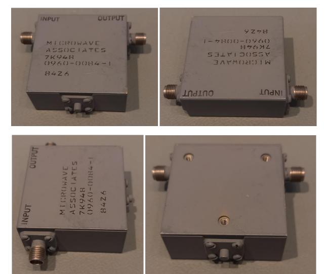
The isolator is housed in a solid metal case and has female SMA connectors at the input and output port.
