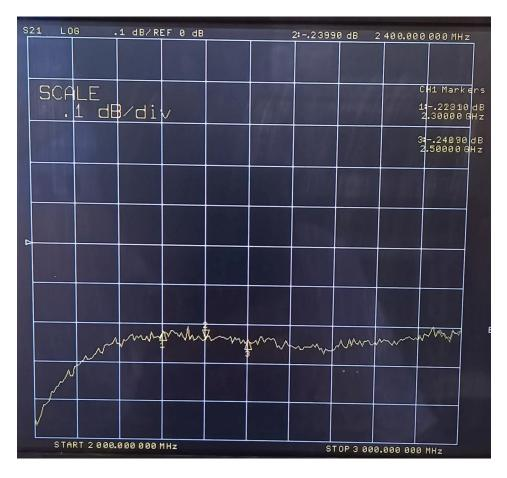
S12 reverse transmission / isolation at 2400MHz is 22.7dB
