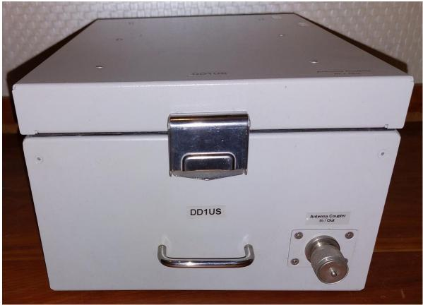
During noise measurements the noise source is placed inside the shielded box and its pulsed 28V DC supply voltage is supplied via a BNC feedthrough connector. Outside of the shielded box I use an additional LC-lowpass filter in another small shielded box in order to additionally filter the pulsed DC supply signal. I am using this filter also when measuring noise figures outside of the shielded chamber.
