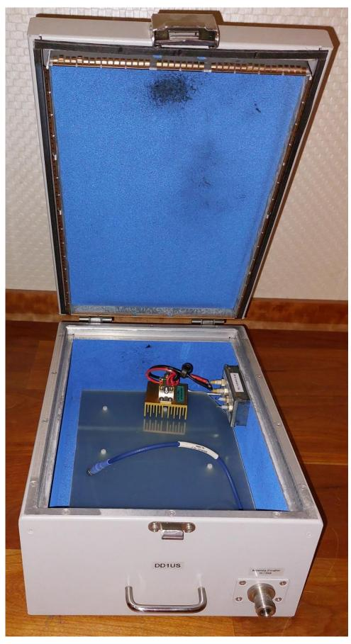
If not all RF feedthrough connectors are needed during a measurement, I am screwing shielding caps on the unused RF jacks.
