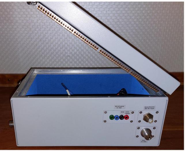
Especially for noise measurements I can add a low noise amplifier inside the box and therefore I can also use longer cables from the output of the DUT to the spectrum analyzer / test receiver.
