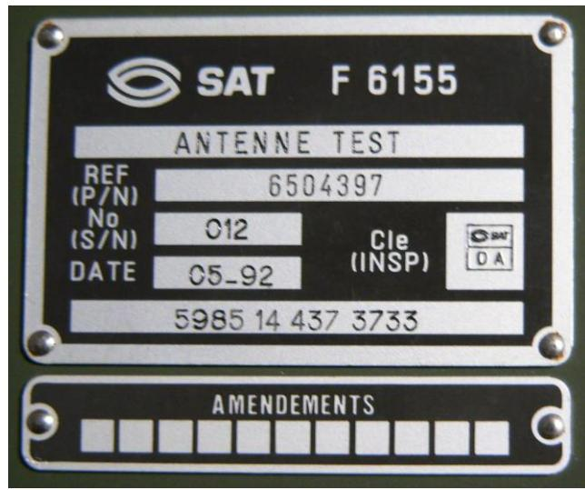
The label suggests that this “ANTENNE TEST” or “F 6155” was built in May 1992. The Logo stands for the SAGEM group, SAT stands for a division of SAGEM which was acquired by SAGEM in 1939. The part number P/N is 6504397. The code “5985 14 437 3773” seems to be a NATO NSN number with “5985” identifying “transmitter and receiver”.
