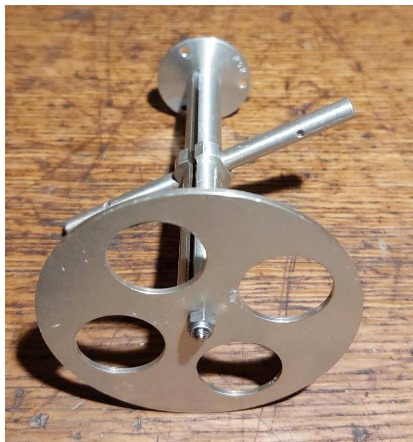
Interestingly the combined length of both dipole antenna elements is shorter than the diameter of the reflector disc. It is also unclear to me why a disc is used as the feed is linear polarized and simple aluminium bar for the reflector would be sufficient.
