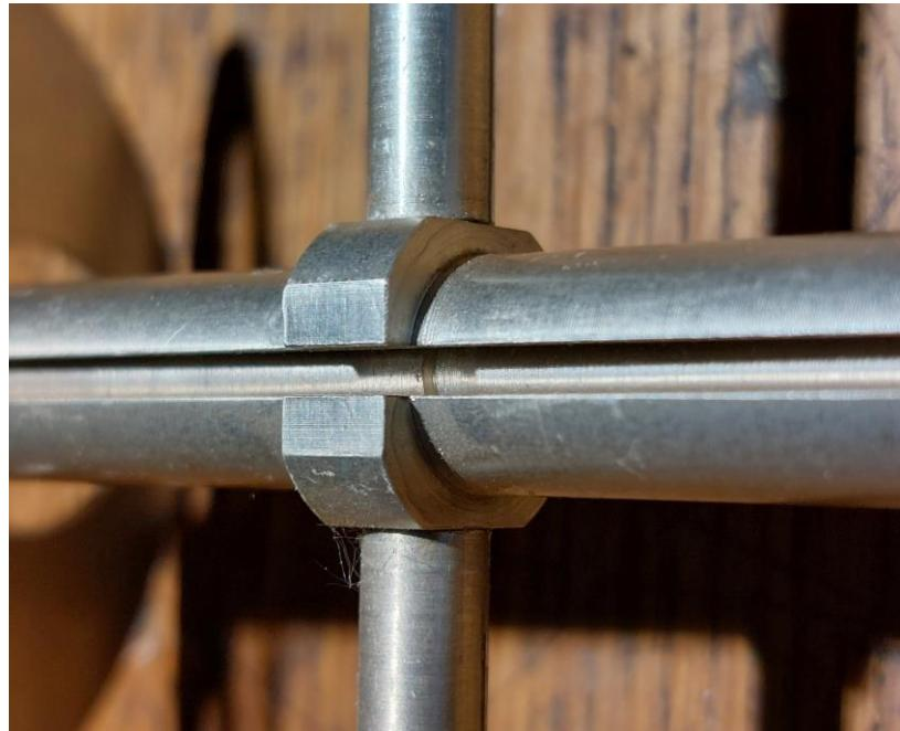
The section of the slotted line between the location where the dipole elements are attached to the reflector disc has a slightly thicker inner conductor and thus lower impedance than the section between the coaxial SMA connector and the dipoles. The length of both slotted line sections is about 50mm which indicates a possible target frequency of 1.5GHz.
