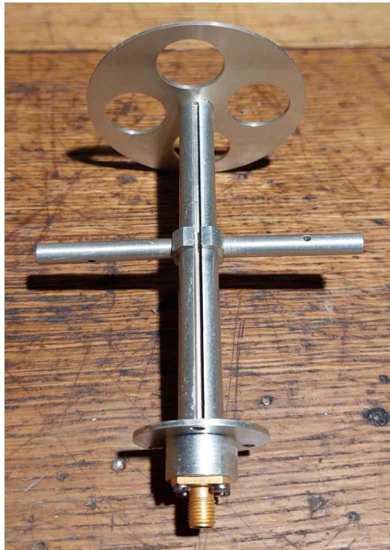
From the coaxial SMA jack to the dipole elements a slotted coaxial line is used which acts as a balun to convert the single ended signal from the coaxial jack to a symmetrical signal for the dipole feeds.
