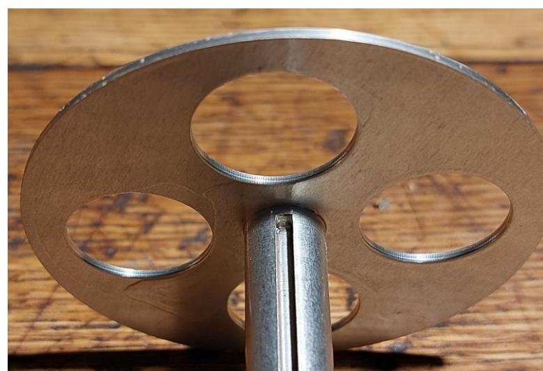
The slotted line is extended to the disc shaped reflector element which is providing also a short between the inner conductor and the outside slotted shield. This is also part of the balun and matching circuit.
