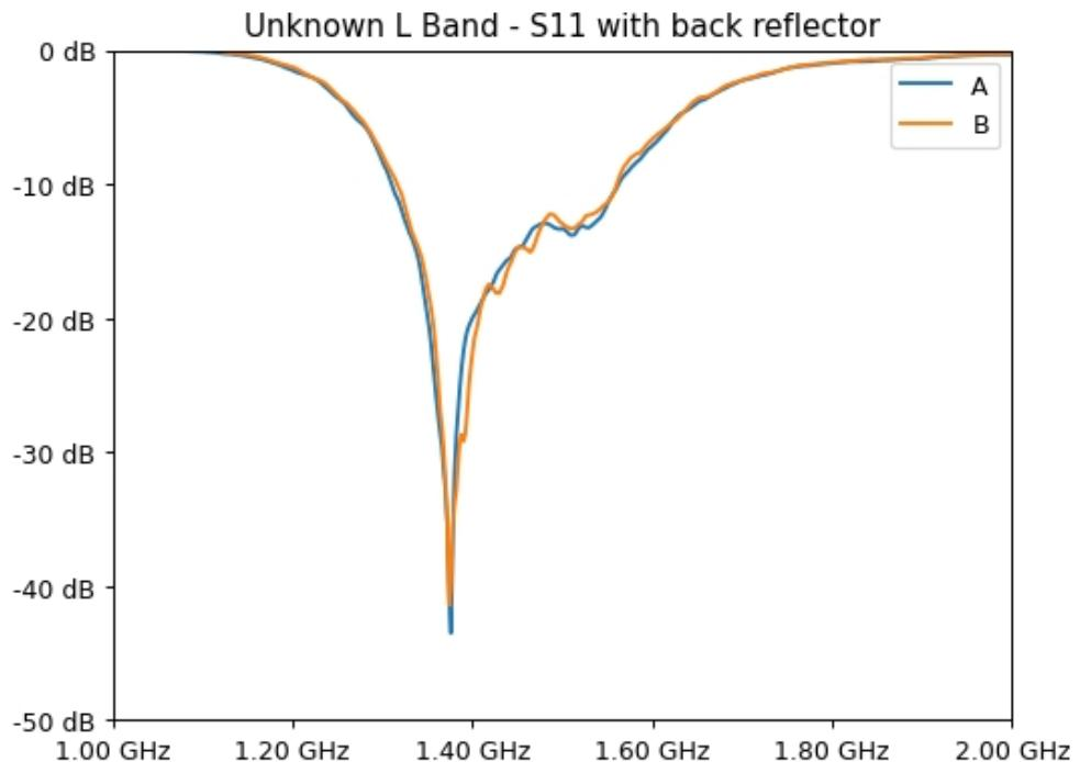
Apparently, the resonance is shifted to below 1.4 GHz when the feed is mounted to a reflector plate.
