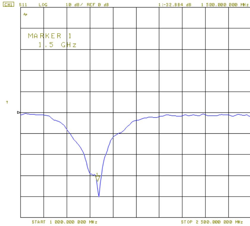
The return loss shows a very distinct optimum at about 1.5GHz. The VNA was not calibrated thus the exact return loss value is unknown but it is at least 30dB. Thus, the initial estimate of the target frequency of this antenna at 1.5GHz matches quite well.
