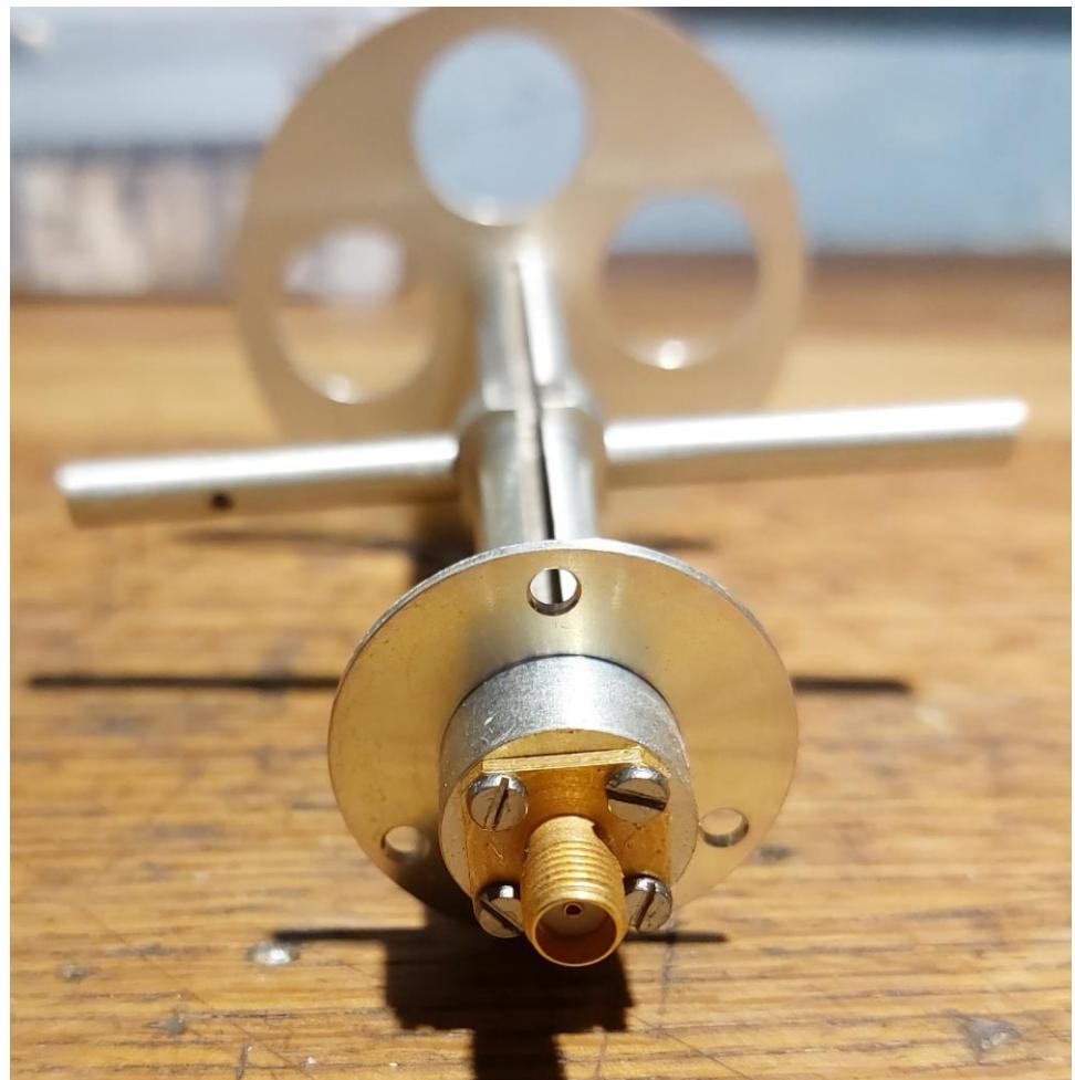
The input connector is an SMA jack. The barrel to which the jack is attached is normally most likely mounted in a reflector plate and fixed with 3 screws though the holes in the round disk.
