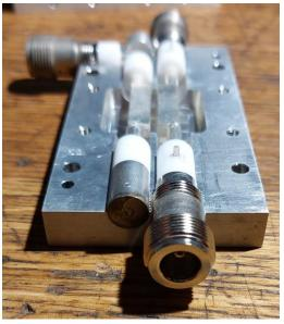
The inside of the coupler looks very professionally made. All parts fit tightly in the milled-out cavities and there are dowel pins which make sure that everything fits perfectly during assembly.
