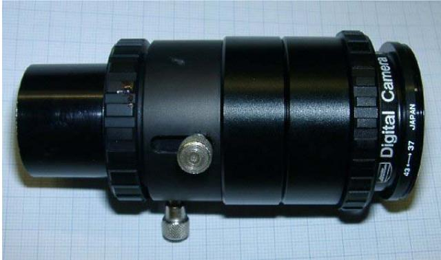
Fig. 1: Eyepiece projection adapter incl. Casio adapter
