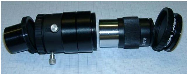
Fig. 2: Eyepiece projection adapter disassembled
