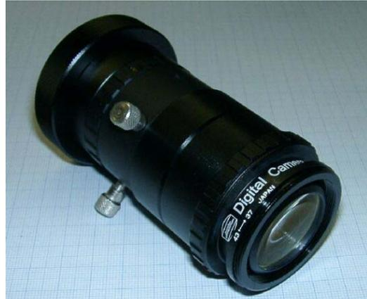
Fig. 5: OPFA-3 with 25mm Plössl eyepiece
