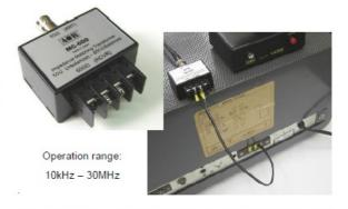
MC-600 is an optional interface between the 600 $\Omega$  antenna socket of your antique radio, and the 50 $\Omega$  input of the LA390 (or LA380) loop antenna. Supplied with a 30cm lead terminated with solderless terminals.
