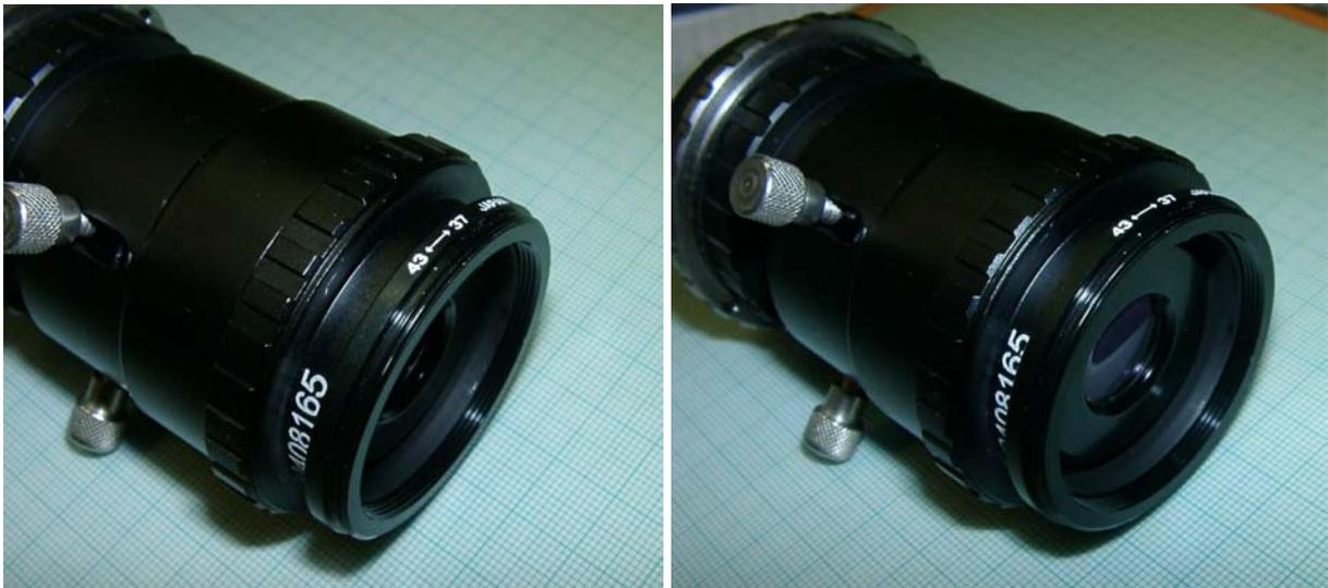
Digi-T-adapter and adapter ring 37mm-43mm. The video camera shall be adapted to the 43mm thread.
