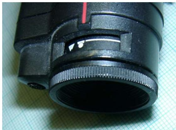
The camera head includes an objective, which can be focused. The objective does feature an inner thread which shall be used to attach an adapter.
