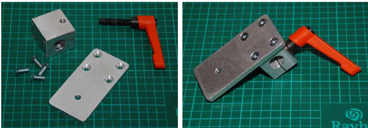
This clamp is moved over the counterweight rod and then fixed with the red handle. On the clamp I mounted a surplus head from a camera tripod to be able to make the necessary fine adjustments of the then to be attached camera.
