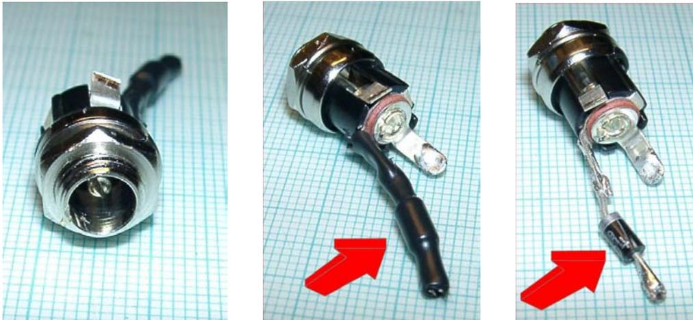
The second diode does protect the telescope from being reverse powered through the "+12V output". This output is the jack on top of the mounting base (with plug inserted).
