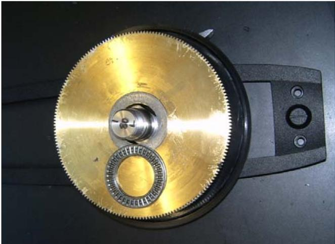
The next few pictures show you the sequence and the parts to be removed to get access to the clutch. First the gear gets off.
