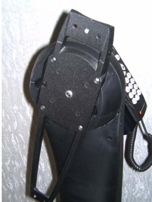
This is the left fork arm with the clutch. To remove it OTA you now see the fork arms like this. To remove it the large nut at the outside of the fork arm needs to be removed. You can then remove the bearing and next separate the holder of the OTA from the fork completely.
