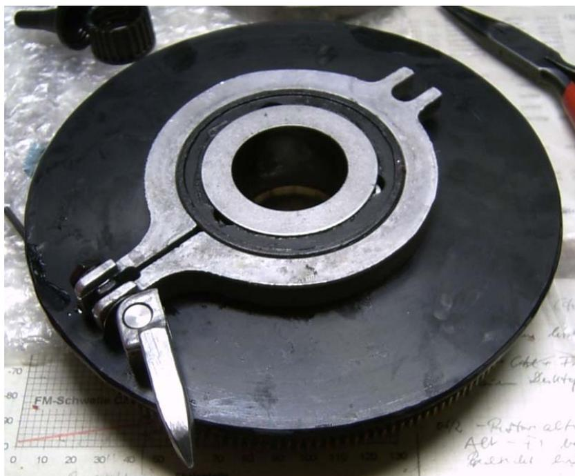
Another point of adjustment is the big nut which we had to remove to disassemble the fork arm. This nut clamps the tapered roller bearings. This type of bearing requires a certain "looseness" to operate correctly. I tightened the nut to the point, where the arm was still rotating freely with no discernable lateral movement of it possible. I also secured the nut with some screw sealing lacquer. The next picture shows the nut and underneath the bearings I am referring to.
