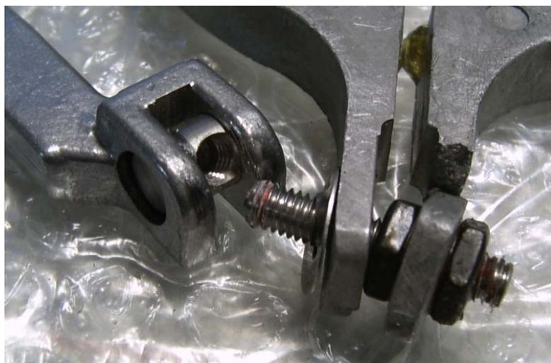
Then you also remove the 3 nuts from the threaded rod (also secured with the lacquer). You should now see the following parts in front of you ...
