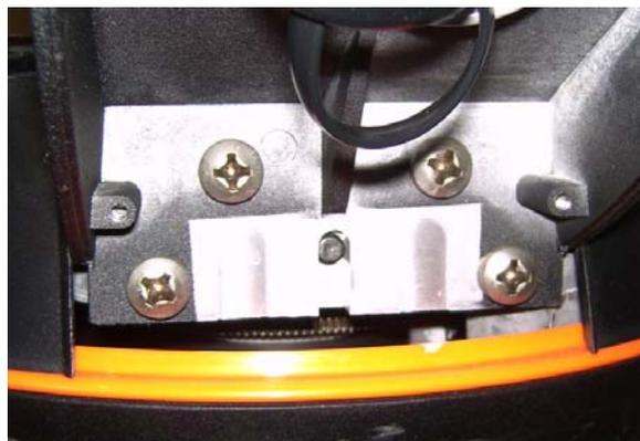
There is one index nose on each of the sides of the OTA – take care not to brake them. Very little power is needed to remove the OTA from the for mount !
