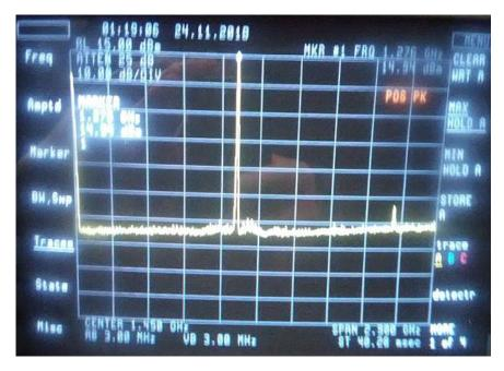
The measured output power at 1270 MHz with 3 MHz RBW is +15dBm. The 2<sup>nd</sup> harmonic at 2540 MHz is approx.. 53dB lower.
