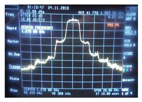
Looking at the signal with the span of the spectrum analyser reduced to 20 MHZ one can see the typical DVB-S2 signal shape. The measurement was done in max. hold mode. The "shoulders" of the DVB-S2 signals are quite high (-25dBc) i.e. the transmitter is not operating linear enough.
